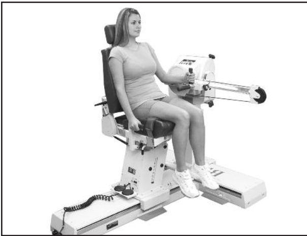
Figure 4.11. Elbow Extension/Flexion. Dynamometer rotation = 0 degrees, Chair rotation = 0 degrees.
