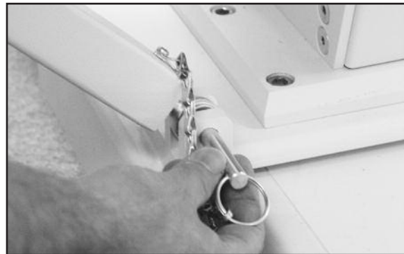
Figure 1.6. Attaching the Seat Back Brace to the Multi-Joint System trolley mount clevis
