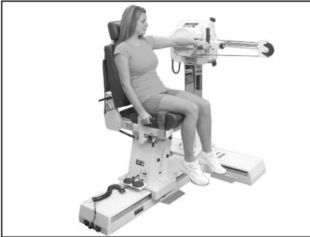
Figure 4.10. Chest Press/Lat Row. Dynamometer rotation = 0 degrees, Chair rotation = 0 degrees.
