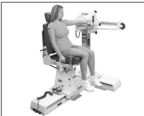
Figure 4.7. The handgrip can be inserted with the neutral handle facing up or down based on patient protocol. Dynamometer rotation = 0 degrees, Chair rotation = 0 degrees.
