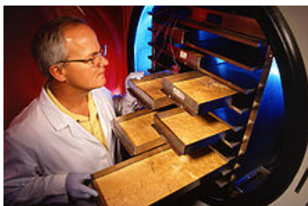
Unloading trays of freeze-dried material from a small cabinet-type freeze-dryer
