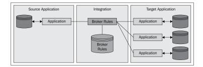
The broker pattern can be broken down into the following logical components:
