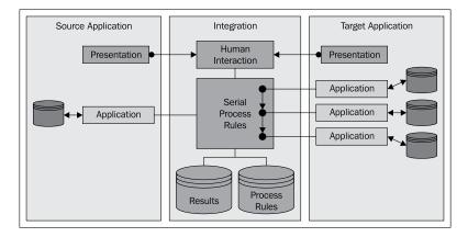
It extends the capability of simple serial process orchestration to include support for user interaction during the execution of individual process steps. As a result, it supports a classic workflow.
