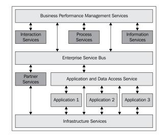
An ESB is used as the central integration component for service calls. It has similar properties to those of the integration platform in hub-and-spoke architecture, or of the bus in pipeline architecture. A SWOT analysis is shown in the following table
