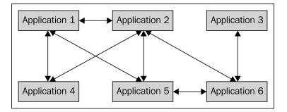
As shown in the above diagram, in this architecture, there is no central database – each system has its own data storage.
