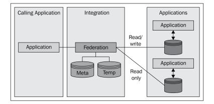
The federation pattern as shown in this diagram can be broken down into the following logical building blocks:
