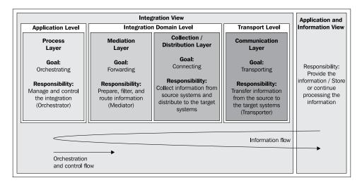
The blueprint allows for this by assigning the four layers shown above to the following three levels:
