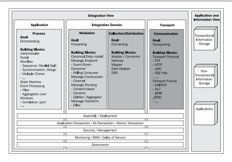
The allocation of the various layers of the Trivadis Integration Architecture Blueprint to the **application**, **integration domain**, and **transport levels**, enables an integration solution to be embedded in an overall architecture. From an application perspective, the management of the information flow as a business process is essential, while standardized and reliable communication is important for the technical infrastructure.
