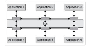
Similarly to the hub-and-spoke architecture, this architecture also keeps interface problems to a minimum. The use of appropriate middleware components allows the communication between the systems to be standardized. The bus system is responsible for message distribution. The transformation and routing rules are stored in a central repository. Depending on the middleware product in use, business functions and rules can also be represented. A SWOT analysis is shown in the following table:
