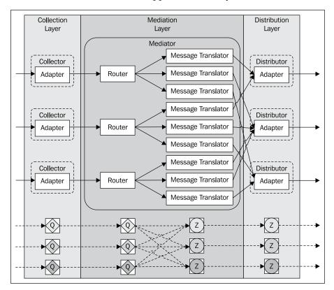
The problem can be resolved by introducing a general format, which is used in the integration solution and in all new target applications. Only one mapping to this internal format needs to be maintained for the existing applications. This keeps maintenance and development costs to a minimum. Internal formats of this kind are referred to as **canonical formats**. In the context of ESB, the term **normalized message format** is also used.
