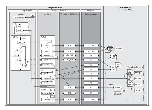
The extraction and file creation logic is written in PL/SQL. A Unix shell script is used to send the files through the **File Transfer Protocol (FTP**), as no direct FTP call was possible in PL/SQL. Both a shell script and the PL/SQL logic are responsible for orchestrating the integration process.
