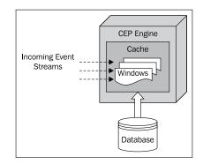
• **Aggregation over windows**: Computes statistics over different types of sliding windows (for example, a time-based window covering the last 10 minutes or an event-based window with the last 10 events).
