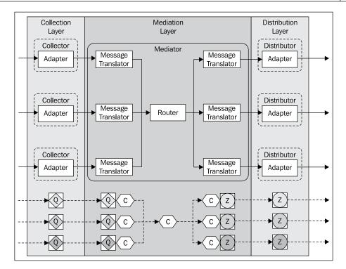
Canonical data models are independent of any specific application. Each application is decoupled from other formats and only needs to be able to generate and read the canonical format. Application-specific components that implement the message translator pattern are used for this purpose.
