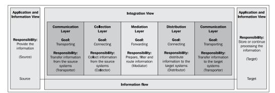
The diagram shows the layers without the optional process layer. In the case of simple information flows, this layer can be omitted. It will be described in a later section.
