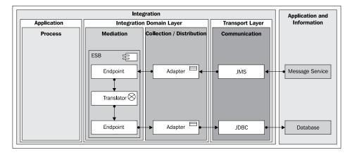
It is clear that an adapter is an object. In an actual implementation, this could be a Java or a .NET object, for example. The ESB building block is shown as a component that contains other building blocks, and among these is the translator building block that is designated as an operation. In an implementation, this can take the form of one or multiple methods of a class or a module (for example, Oracle PL/SQL package).
