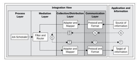
However, the orchestrator in the process layer can also be activated or triggered by a source system, as demonstrated in the following diagram. In this case, the orchestrator role is fulfilled by a workflow or BPEL building block, and by that, implements an integration process.
