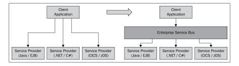
The encapsulation of services by the ESB means that the client application does not need to know anything about the location of the services, or the different communication protocols used to call them. The ESB enables the shared, enterprise-wide, and even intra-enterprise use of services and separate business processes from the relevant service implementations (Lee et al. 2003).
