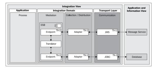
This scenario shows an integration solution which reads from a JMS queue via an adapter in a transaction, transforms the information, and then writes the data via JDBC to a database table (in the same transaction). The source only considers a message to have been processed if it was successfully written to the database table (using an XA transaction), which makes it possible to guarantee reliable transmission.
