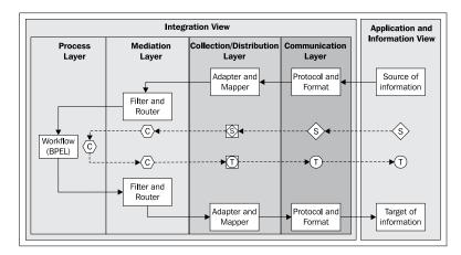
A query or message from an information source initiates the integration process via protocol and format, and through filter and router building blocks. The process is executed autonomously and uses an additional filter and router building block to initiate the target systems.
