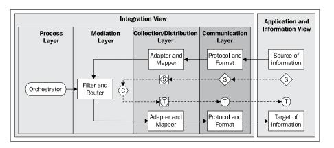
In this case, the orchestrator controls the mediation layer and can therefore start the integration or the information flow, for example. The mediator and the building blocks which implement the mediator functionality become passive entities that are initiated by the process layer.
