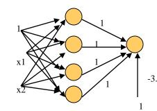
One-hidden layer network that realizes the convex region: Each hidden node realizes one of the lines bounding the -3.5 convex region
