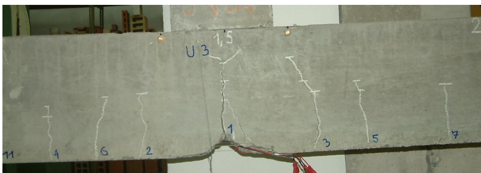
Figure 17. Crack pattern after collapse of beam R50.
