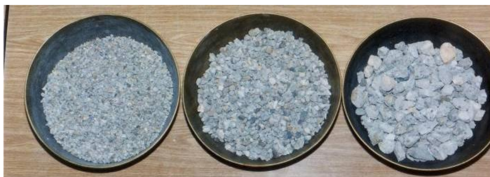
Figure 3. Recycled concrete aggregate fractions. From left to right; 4–8 mm, 8–16 mm and 16–31.5 mm coarse aggregates.
