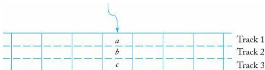
Before introducing other models, we make one remark on the standard Turing machine. It is implicit in [Definition 9.1](#) that each tape symbol can be a composite of characters rather than just a single one. This can be made more explicit by drawing an expanded version of [Figure 9.1](#) ([Figure 10.1](#)), in which the tape symbols are triplets from some simpler alphabet.
