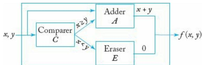
The program for the comparer  $C$  is written as suggested in [Example 9.11](#), using a Turing machine having states indexed with  $C$ . For the adder, we use the idea in [Example 9.9](#), with states indexed with  $A$ . For the eraser  $E$ , we construct a Turing machine having states indexed with  $E$ . The computations to be done by  $C$  are
