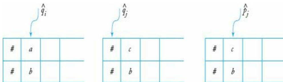
Sequence of configurations in simulating  $\delta(q_i, a) = (q_j, c, L)$ .
