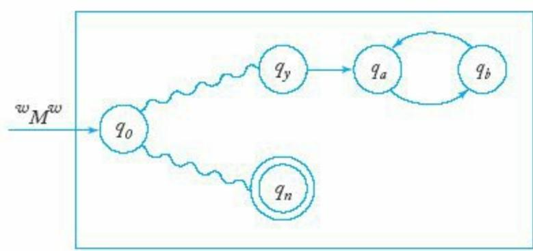
From  $H$  we construct another Turing machine  $\hat{H}$ . This new machine takes as input  $w_M$  and copies it, ending in its initial state  $q_0$ . After that, it behaves exactly like  $H$ . Then the action of  $\hat{H}$  is such that
