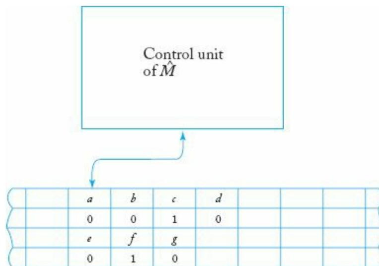
The simulation of an off-line machine  $M$  by a standard machine  $\widehat{M}$  requires a lengthier description. A standard machine can simulate the computation of an off-line machine by using the four-track arrangement shown in [Figure 10.7](#). In that picture, the tape contents shown represent the specific configuration of [Figure 10.6](#). Each of the four tracks of  $\widehat{M}$  plays a specific role in the
