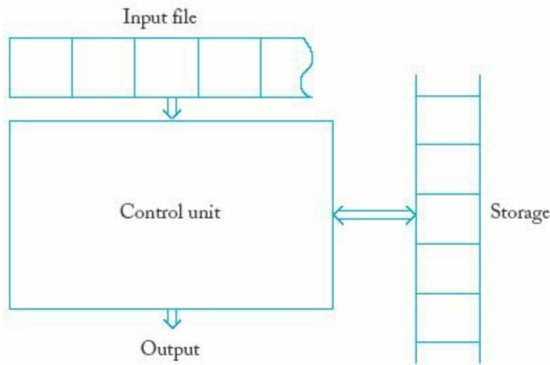
This general model covers all the automata we will discuss in this book. A finite-state control will be common to all specific cases, but differences will arise from the way in which the output can be produced and the nature of the temporary storage. As we will see, the nature of the temporary storage governs the power of different types of automata.
