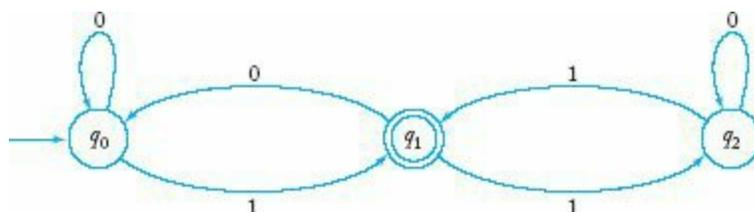
It is convenient to introduce the extended transition function  $\delta^* : Q \times \Sigma^* \rightarrow Q$ . The second argument of  $\delta^*$  is a string, rather than a single symbol, and its value gives the state the automaton will be in after reading that string. For example, if
