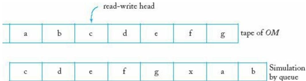
A right move is easy, as we just remove the front symbol in the queue and place something in the back. A left move, however, goes against the grain, so the queue contents have to be circulated several times to get everything in the right place. It helps to use additional markers  $Y$  and  $Z$  to denote boundaries. For example, to simulate
