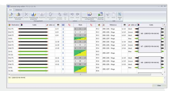
The Terminal Strips Editor can be used to create wiring terminals, renumber terminals, and manage multi-level terminals.
