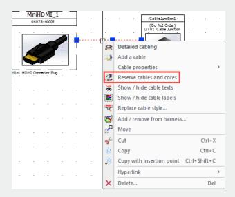
This options access the Cables and Cores Reservation dialog where cables can be reserved and then used later in the schematic design development.
