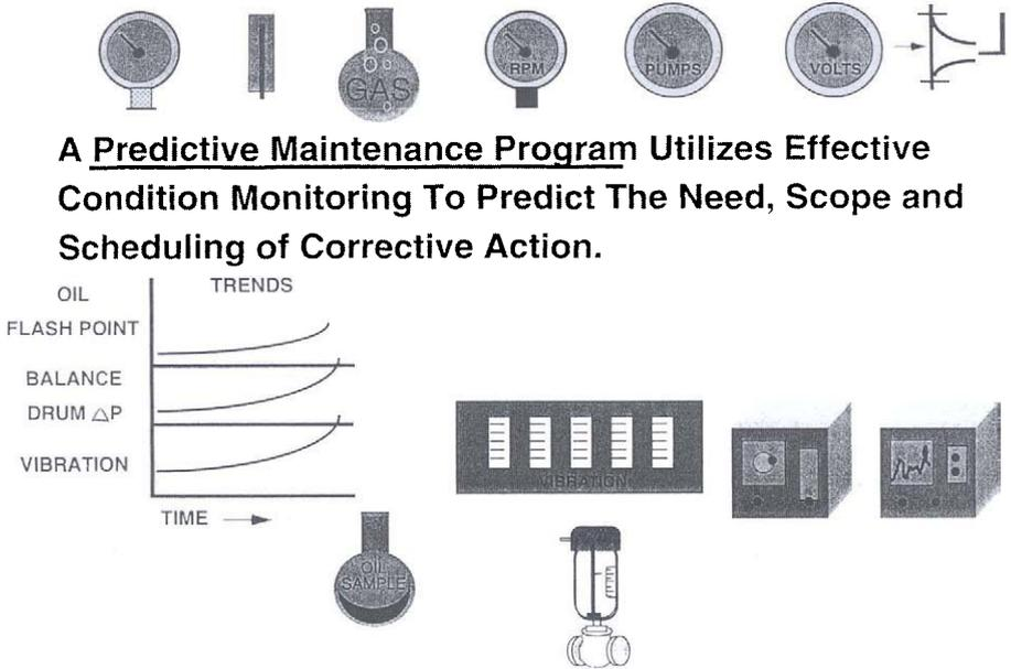
Figure 3.9 A predictive maintenance program (Courtesy of M.E. Crane Consultant)
