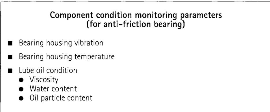
Figure 3.6 Component condition monitoring parameters (for anti-friction bearing)
