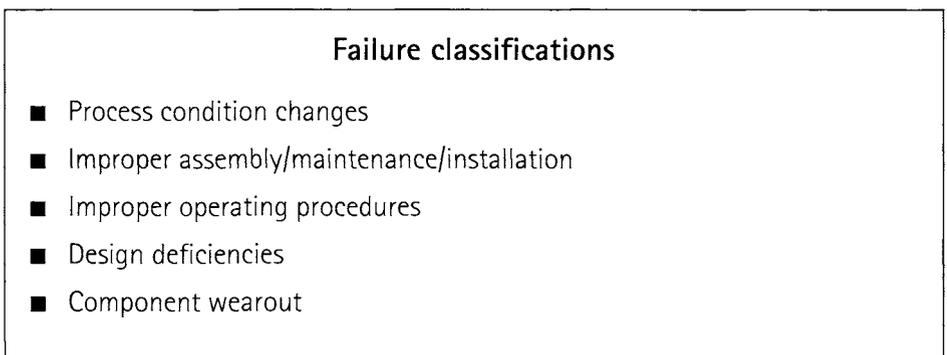
Figure 3.1 Failure classifications
