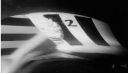
Fig. 6.11. Cavity at the impeller blade leading edge
