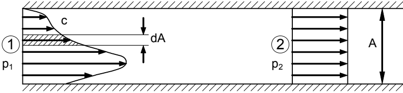
Fig. 1.16. Equalization of a non-uniform velocity distribution
