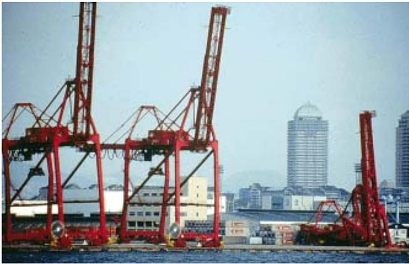
*Cranes damaged by lateral spreading, Rokko Island.*
