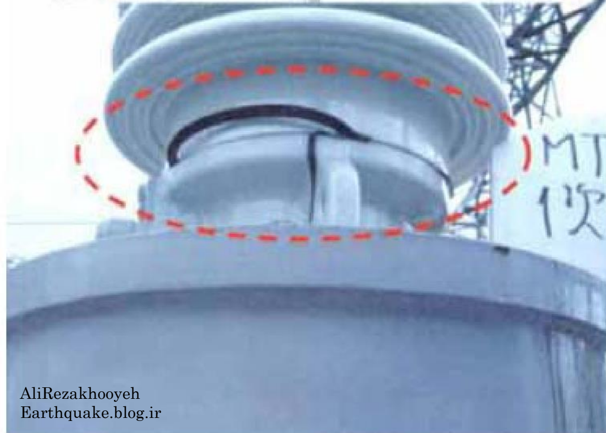
Figure 4 Extrusion of gasket and oil leakage in bushing of 154 kV transformer in Uonuma Sub. (JSCE, 2004)
