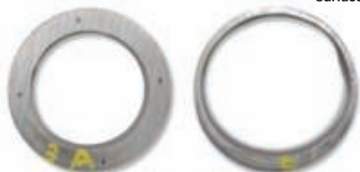
FIGURE 2. Tubewall thinning is caused by single-phase FAC
