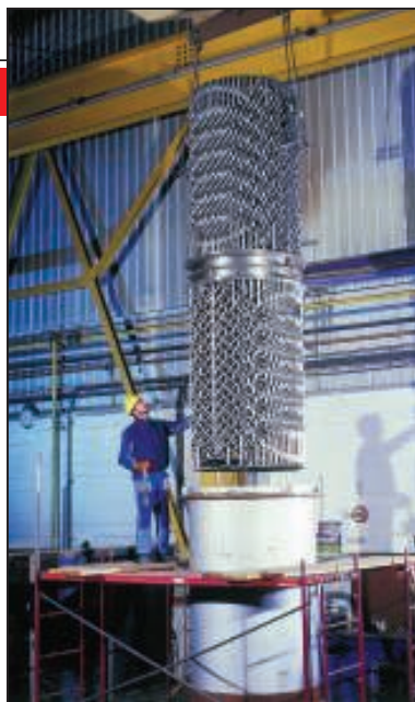
FIGURE 3. The Sulzer Mixer Reactor (SMR) is a tube-bundle heat exchanger that allows high-effective cooling or heating of viscous media. The SMR is a suitable choice to combine effective mixing with controlled heat transfer
