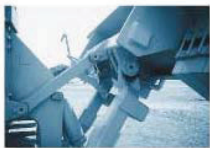
Some slender pin-connected members used in moving machinery, such as this short link, are subjected to compressive loads and thus act as columns.
