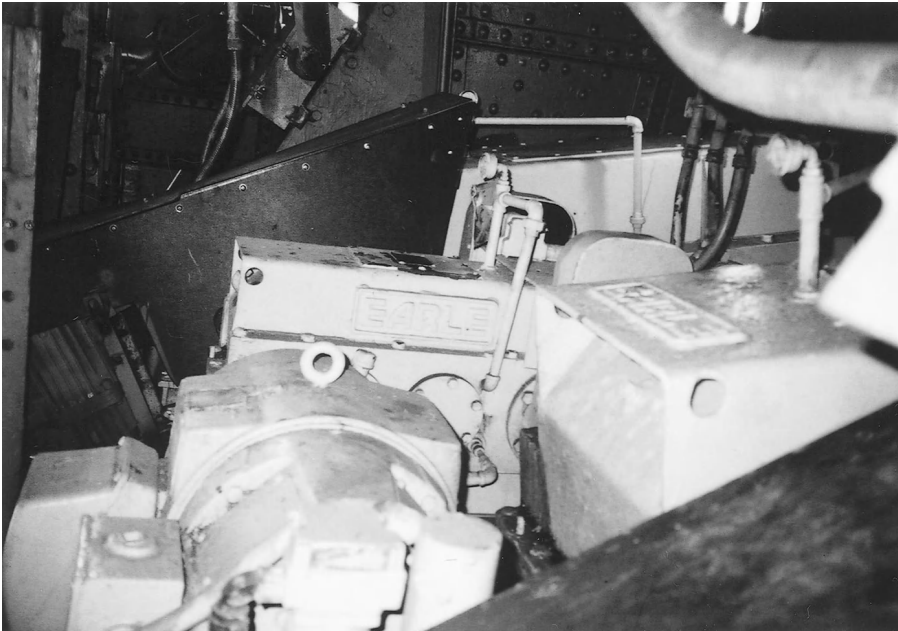
Figure 17-12 Parallel Shaft Differential Reducer. The gearbox in the center of the picture, behind the motor that powers it, delivers drive torque equally to the two secondary reducers, one to the right in front, and the other behind.
