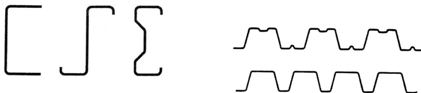
Figure 1.11 – Cold formed sections
