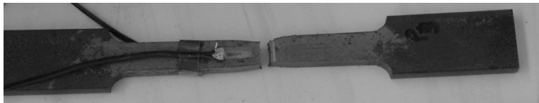
Figure 1.6 – Geometry of proportional flat test samples
