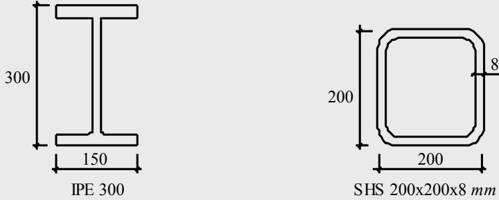
Figure 2.84 – Classification of cross sections
