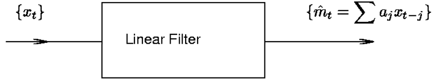
Figure 1-20 Smoothing with a low-pass linear filter.
