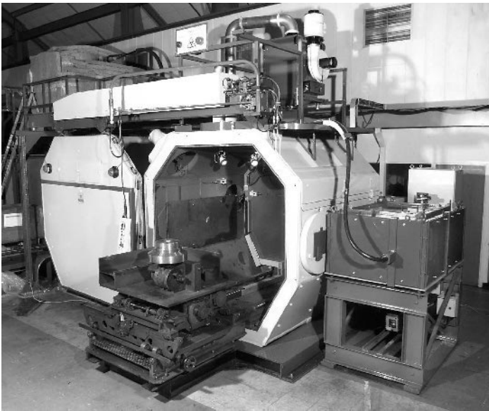
8.8 A 2 m 3 chamber, 100kW, electron beam welding machine, showing the open vacuum chamber. It is capable of welding up to 200mm thick aluminium. Courtesy of TWI Ltd.
