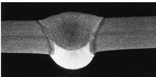
6.5 AC-TIG argon shielded (a) unbacked 3mm sheet, single pass, flat position; (b) unbacked 6mm thick plate, two pass, flat position.
