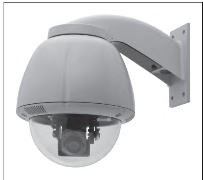
FIGURE 17-13 Outdoor pan/tilt dome configuration
