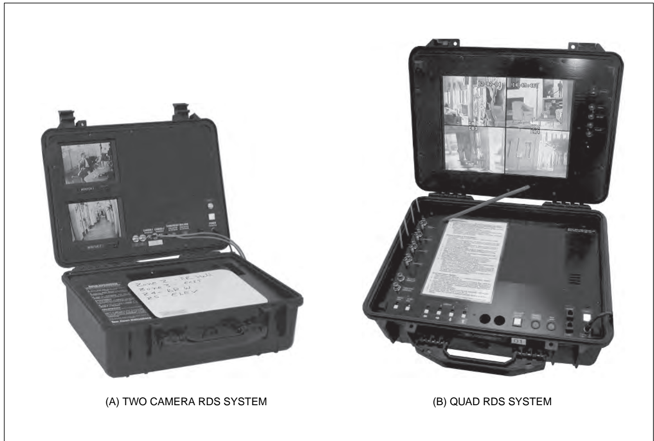
FIGURE 21-2 Typical rapid deployment security (RDS) systems with wired and wireless video monitoring
