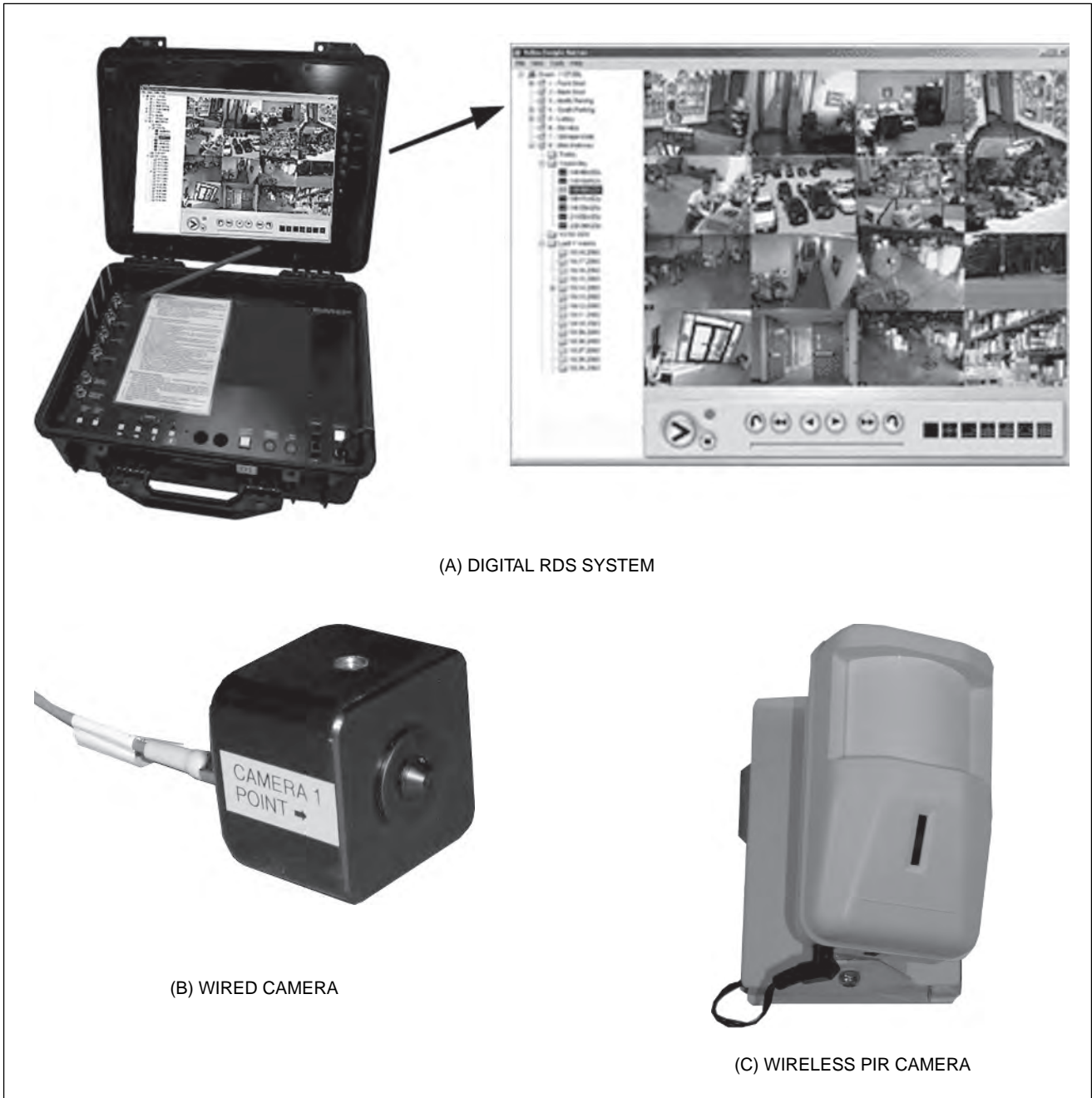
FIGURE 21-4 Typical digital rapid deployment system with wired and wireless video
