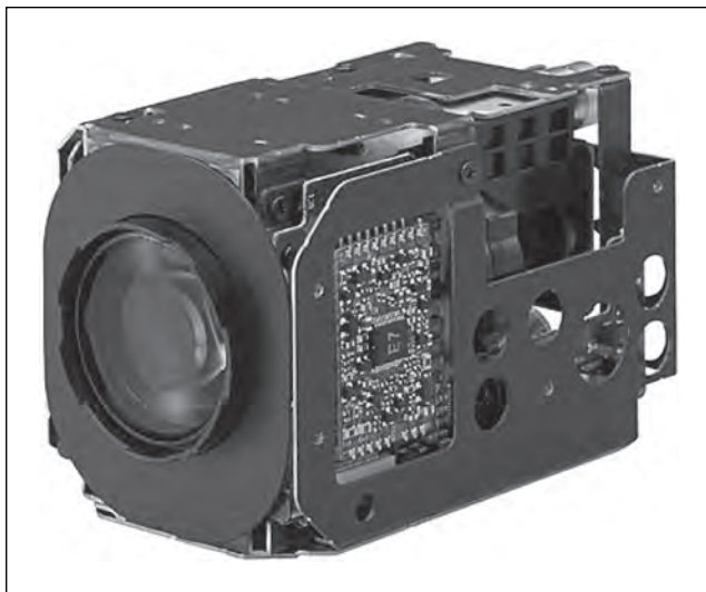
FIGURE 4-26 Compact zoom lens–camera cube
