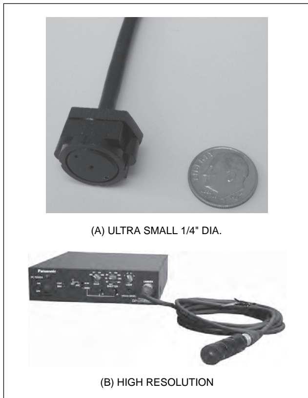
FIGURE 18-20 Remote head cameras
