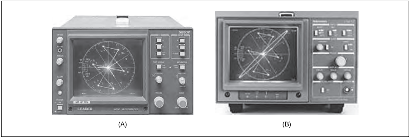
FIGURE 25-6 Vectorscope for calibrating color video equipment
