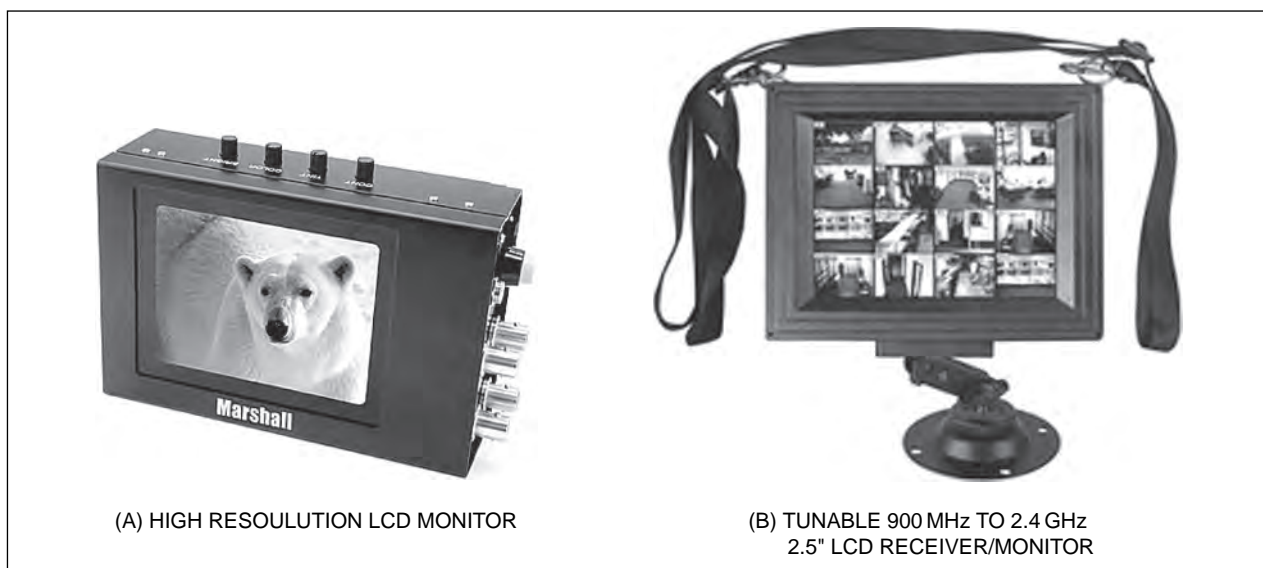
FIGURE 8-16 Small flat screen receiver/monitor
