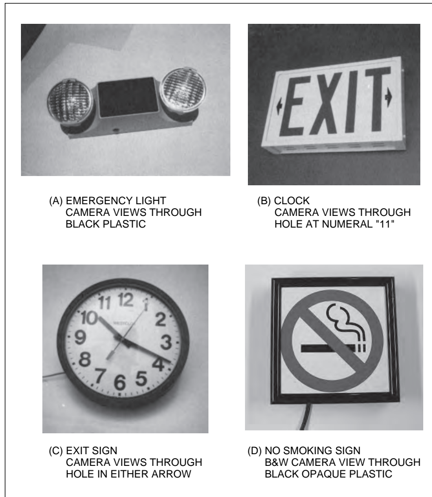
FIGURE 18-21 Covert cameras installed in office building fixtures
