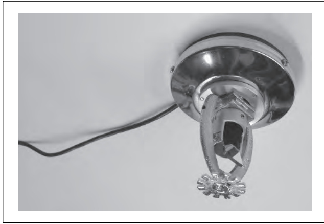
FIGURE 18-24 Sprinkler-head covert camera
