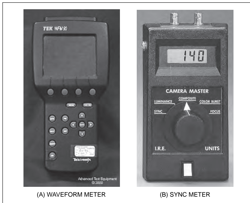
FIGURE 25-13 Hand held video signal waveform and sync signal meters
