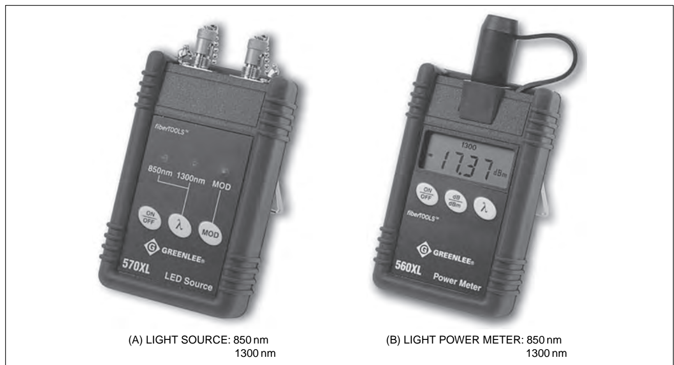
FIGURE 25-21 Fiber-optic light source and light transmission test equipment
