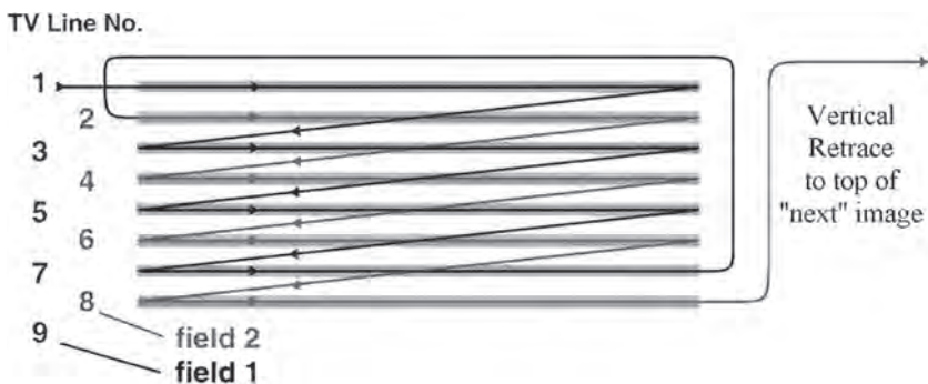
Figure 1-3 Horizontal and Vertical Retrace
