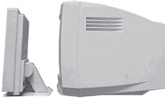
Figure 10-2 LCD Monitor and CRT Monitor Compared
