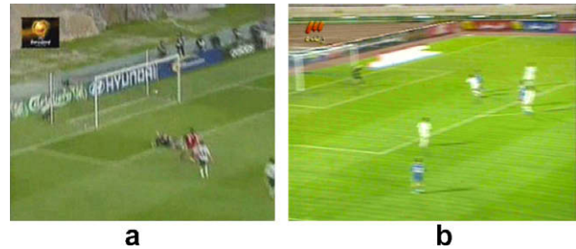
Fig. 10. Some of the samples in which the proper lines could not be detected by our system. The lines are blurring due to fast camera movement and all of them are difficult to be detected (In these samples, some horizontal lines are not detected by our algorithm).
