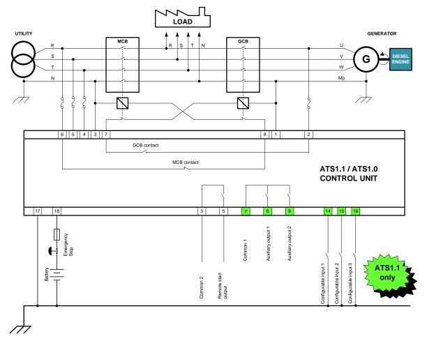
Typical connection diagram is shown above for both models. ATS1.1 has additional auxiliary ports for more specific applications. All ports are configurable through the system menu.
