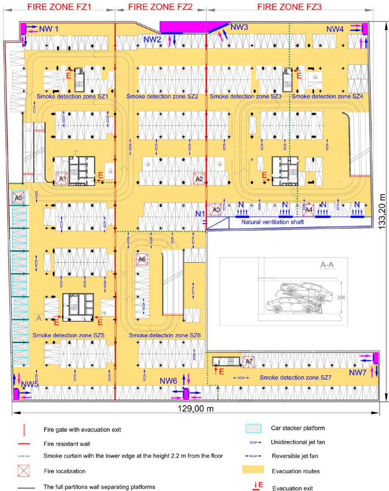
Figure 5. Diagram of the car park and the ventilation system – storey „-2” (repeatable storey). CASE 2A – unsprinklered, with compartmention
