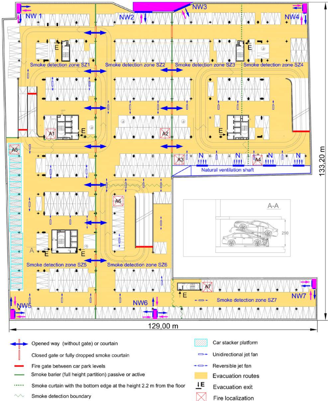
Figure 6. Diagram of the car park and the ventilation system – storey „-2” (repeatable storey). CASE 1B - sprinklered
