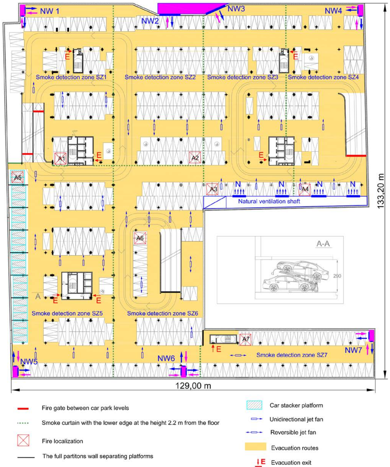
Figure 4. Diagram of the car park and the ventilation system – storey „-2” (repeatable storey). CASE 1A unspinklered, without compartmentation
