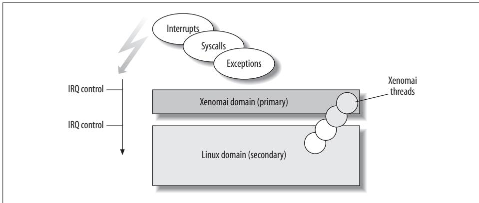
Figure 13-6. Dual kernel support for real-time tasks
