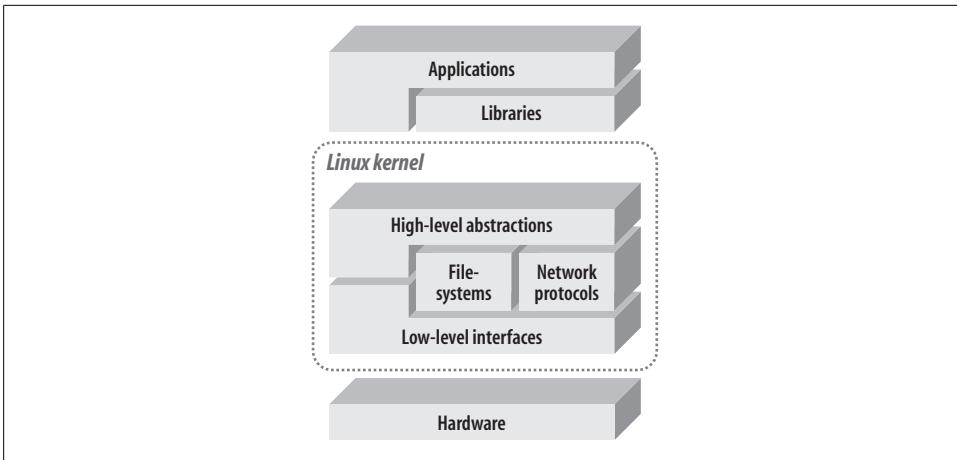
Figure 2-4. Architecture of a generic Linux system
