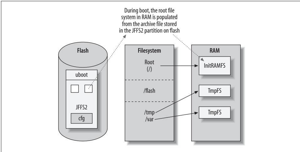
Figure 8-2. Fail-safe upgrade of a RAM-based root filesystem
