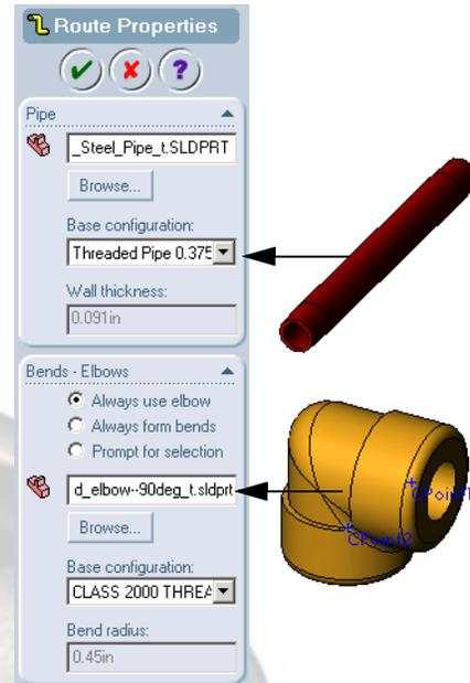
**Note** After adjusting the **Library folder path**, it is a good idea to reload the part files (tube, pipe and elbow) via the **Browse...** buttons to insure that the correct source file is displayed and loaded.
