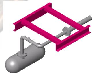
Four commands, **Edit Part**, **Edit Assembly**, **Edit Sub-assembly** and **Edit Route** are used to switch back and forth between editing one component in an assembly and editing the assembly itself. When you are in edit part mode, you have access to all the commands and functionality the part modeling portion of SolidWorks. Plus, you have access to other geometry in the assembly.
