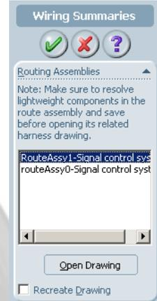
A new drawing file, **RouteAssy1-Signal control system-1.SLDDRW**, is created and saved automatically.
