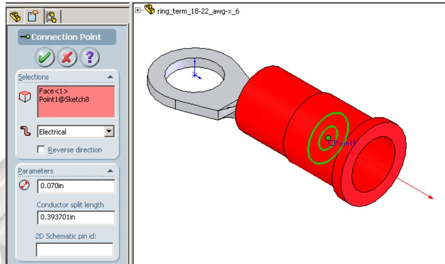
This is a single wire connector, so there is no reason for a Schematic pin id. For connectors with multiple contacts or pins, it may be desirable to add a CPoint for each and index them for individual wire assignments.
