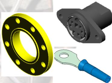
**Assembly Fittings** is a general classification of *assembly* components that are *not* added to the route automatically like pipes and elbows. These include valves, switches and other multiple-part route components.
