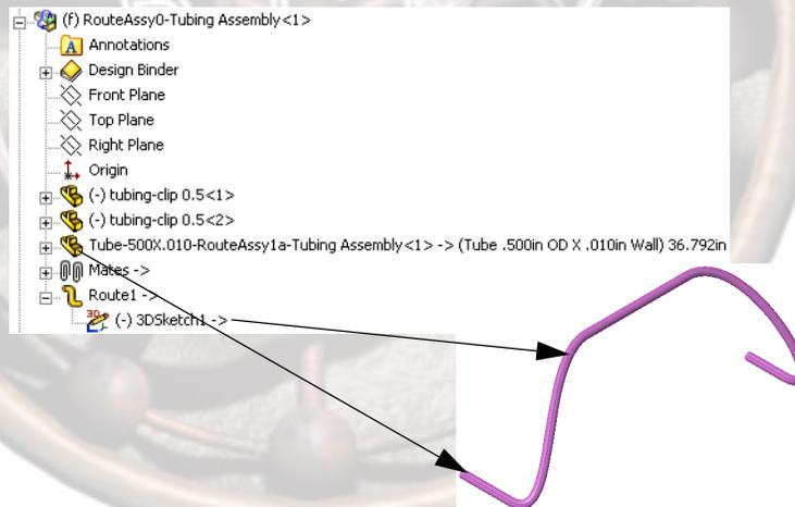
The tube is Tube-500X.010-RouteAssy0-Tubing Assembly with the configuration Tube .500in OD X .010in Wall. The length of the tube is listed following the configuration.
