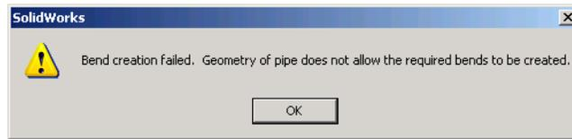
For example, when there is not enough space between two perpendicular segments to put in a full radius of the default size, the segments will show as a sharp corner. An adjustment to that particular radius or to the separation will be needed to show a proper radius.
