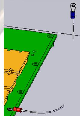
The system auto routes a spline between the terminals. **OK** the Auto Route dialog, and exit the sketch.
