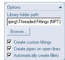
For **Pipe**, choose Threaded\_Steel\_Pipe\_t and **Base configuration** Threaded Pipe 0.375 in, Sch 40.
