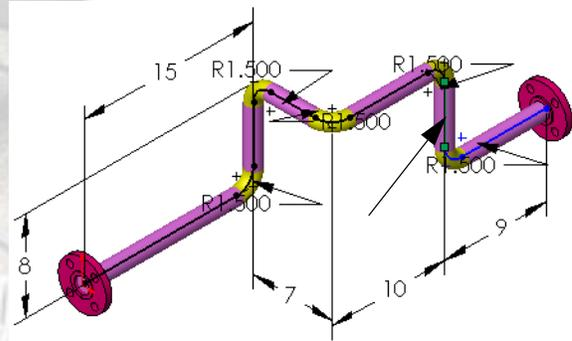
The line, and associated pipe, has been removed from the route.
