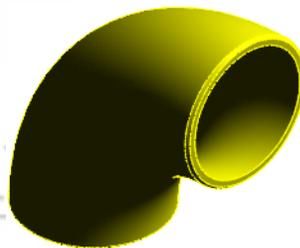
**Custom Elbows** are used where the change in direction is less than 90 degrees but not 45. The system will prompt you to allow the modification of a standard elbow to match the angle. The FeatureManager listing includes name, configuration and sizing.
