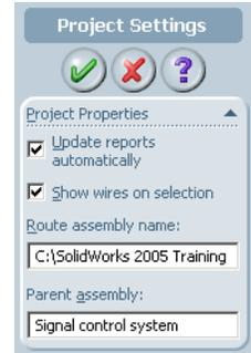
Selection of endpoints will then display what wires are present at that connector endpoint.
