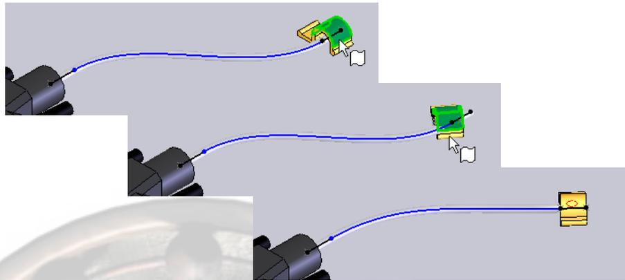
Additionally, if a later **Add Wires** operation changes the size of the route beyond the capacity of the clip, properly size-configured clips will update accordingly.
