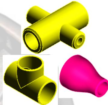
**Flanges and Connectors** are special part fittings that generally connect to both the route and equipment *outside* the route. Because of this, flanges and connectors generally contain **Mate References** for equipment connections.
