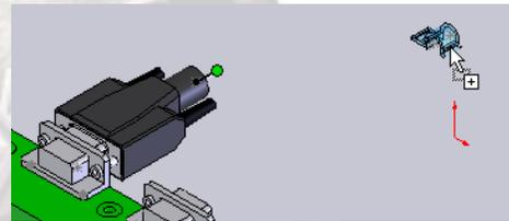
Drag it over the hole in the bottom of the enclosure that's just behind the connector.
