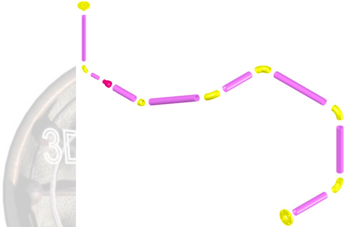
Anywhere the **Fabricated Pipe** changes direction is considered an elbow and is generally represented in the sketch as an arc. The straight lengths are represented as lines.
