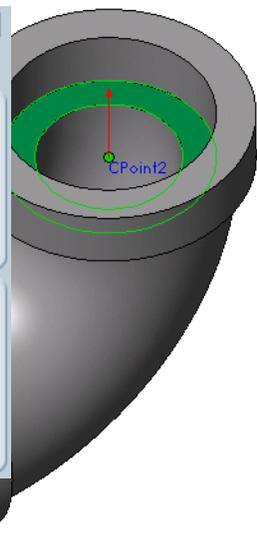
Add another CPoint at the lower connection point. Double-clicking the feature displays the nominal diameter at the connection point.
