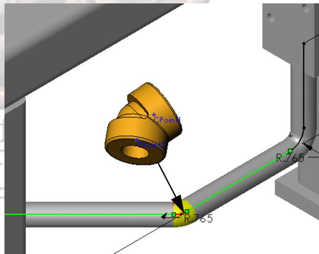
Use **Browse** to select the threaded\_elbow--45deg\_t component for use at this corner. Select the CLASS 2000 THREADED ELBOW, .750 IN as the configuration to use and click **OK**.
