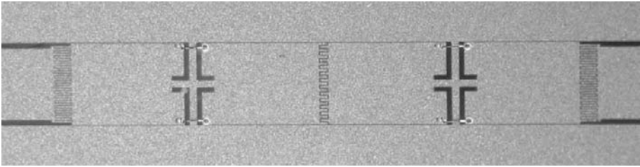
Figure 10: Example of a fabricated CRLH TL.
