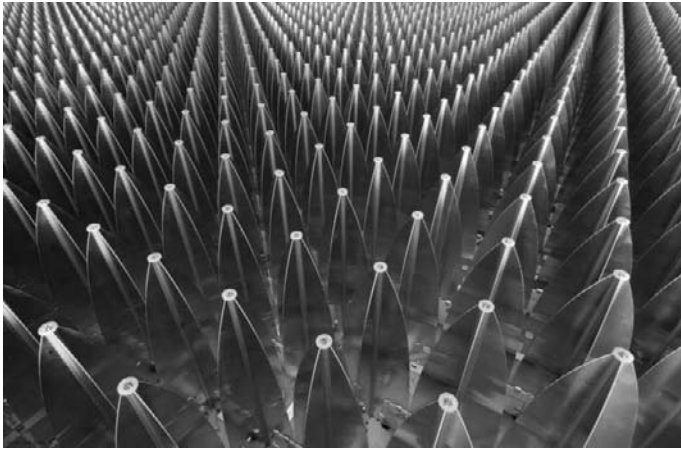
Figure 5: The EMBRACE tapered slot antenna array.
