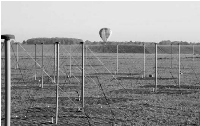
Figure 3: LOFAR Low Band Antennas in a pseudo-random sparse configuration.
