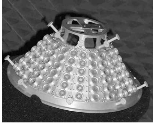
Figure 3: transmission antenna for a spun satellite at L2 Lagrange point (Courtesy of Thales Alenia Space France).
