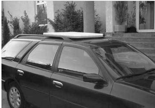
Figure 1: Hybrid rooftop antenna by RaySat Inc. for DBS-reception [1].
