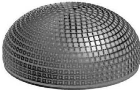
Figure 3: Full electronically steerable array for aeronautical platforms by Space Engineering Spa [2].
