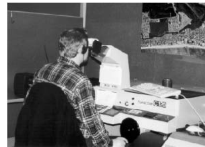
Figure 9-1. Typical analytical stereoplotter (courtesy of Surdex Corporation)
