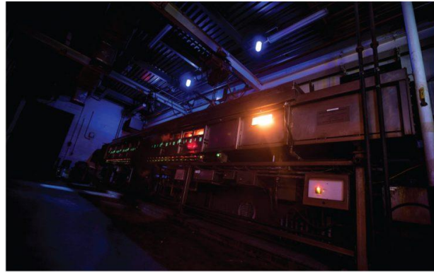
Steiner Tunnel Apparatus—Used for UL 723/ASTM E84 for Insulation Products © UL LLC
