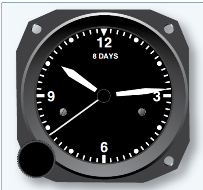
A typical mechanical 8-day aircraft clock.
