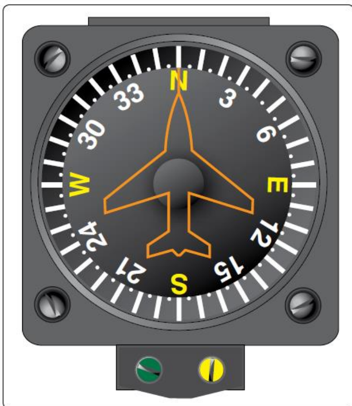
A vertical magnetic direction indicator provides a realistic reference of headings.
