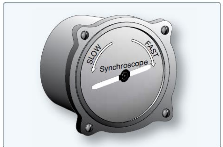
This synchroscope indicates the relative speed of the slave engine to the master
