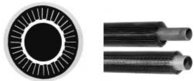
Figure 10-4A(3). Longitudinal fins resistance welded to tubes. The welding of the fins integral to the parent tube ensures continuous high heat transfer efficiency and the absence of any stress concentrations within the tube wall. (Used by permission: Brown Fintube Co., A Koch® Engineering Co., Bul. 80-1.)
