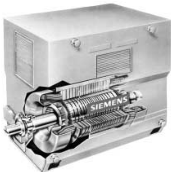
Figure 14-2D. Large horizontal induction motor. Motors can meet API 541 requirements and ISO 9001 Certification for petroleum and chemical industry applications. (Used by permission: Bul. M&DD 3226-3. Siemens Corporation, Motors and Drives Division.)
