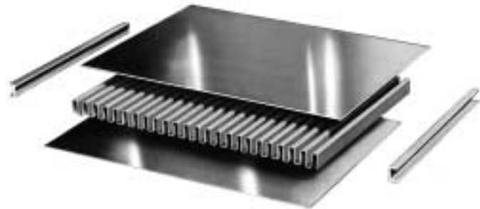
Figure 10-10F. Flat plate extended surface used in low-temperature gas separation plants; exploded view of brazed surfaces. (Used by permission: The Trane® Co., La Crosse, Wis.)
