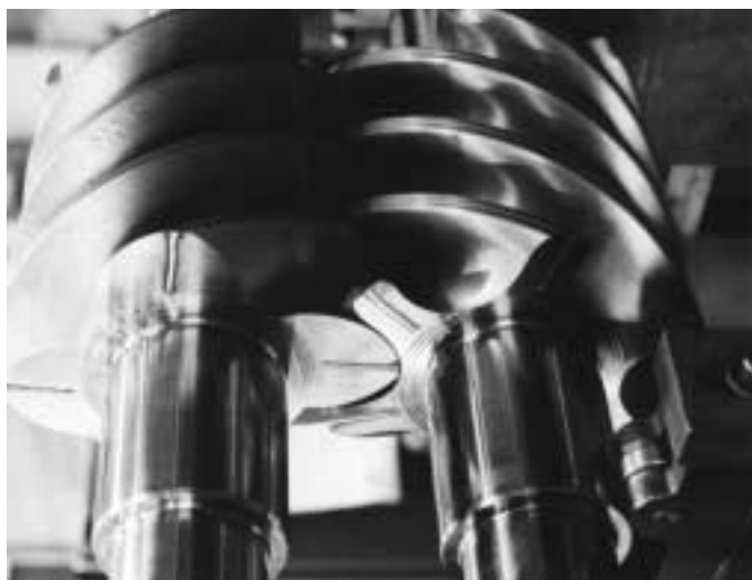
Figure 12-110D. Rotor set for oil-free rotary screw compressor. (Used by permission: Bul. CCB-0057-3-295. A C Compressor Corporation.)
