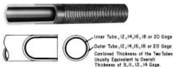
Figure 10-11. Duplex tube. Note inside liner is resistant to tube-side fluid and outer finned tube is resistant to shell-side fluid. (Used by permission: Wolverine Tube, Inc.)
