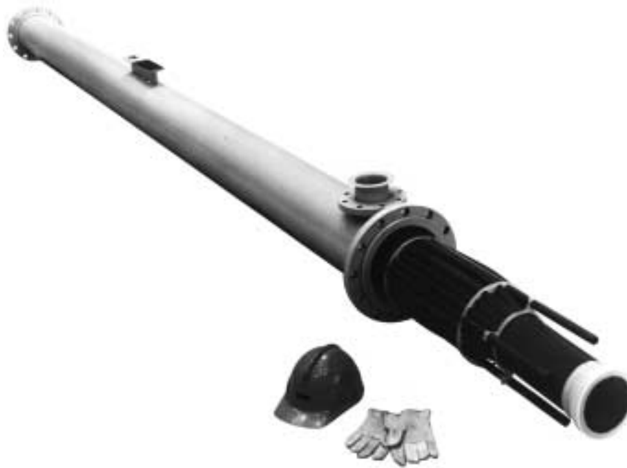
Figure 10-8. Single-pass shell and tube Teflon® tube heat exchanger, countercurrent flow. Tube bundles are flexible tube Teflon® joined in integral honeycomb tubesheets. Shell-side baffles are provided for cross-flow. Standard shell construction is carbon steel shell plain or Teflon (LT)® lined. Heads are lined with Teflon®. Tube diameters range from 0.125–0.375 in. O.D.; the temperature range is 80–400°F; pressures range from 40–150 psig. (Used by permission: AMETEK, Inc., Chemical Products Div., Product Bulletin “Heat Exchangers of Teflon®.”)
