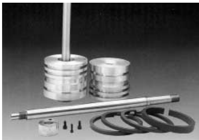
Figure 12-8A. Piston rings. The piston rod is manufactured from heat-treated stainless steel and is coated with wear-resistant overlays, such as ceramic, chromium oxide, and tungsten carbide applied by plasma techniques. Piston rod cross-head attachment has mechanical preloading system for the threads. Rider rings and seal rings are manufactured from PTFE filled resins; fillers are matched to the gas, piston speed, and liner specifications. Typical fillers are glass, carbon, coke, or ceramic. (Used by permission: Bul. BCNA-3P100. Howden Process Compressors Incorporated. All rights reserved.)
