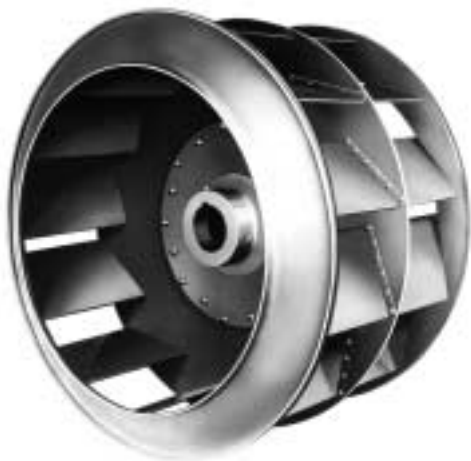
Figure 12-120C. Double-inlet, double-width wheel, backward blades. (Used by permission: The Howden Fan Company.)
