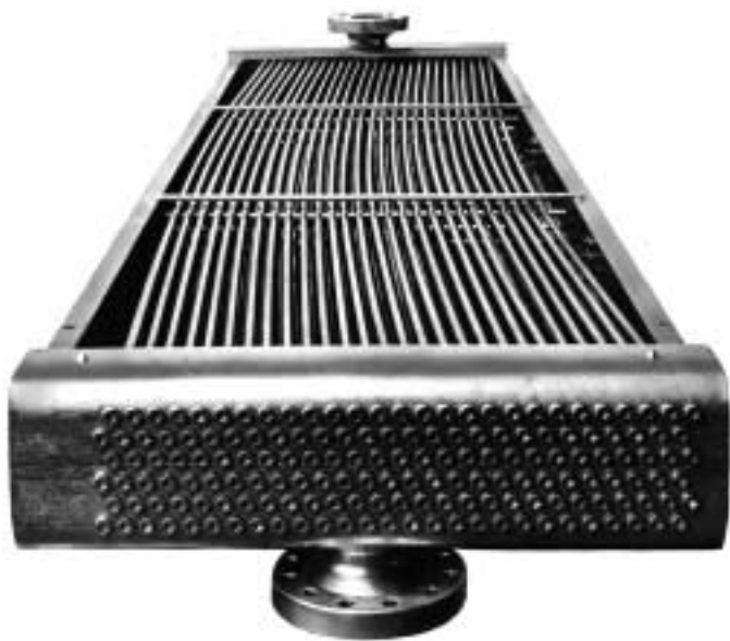
Figure 10-6. Open tube sections. (Used by permission: Griscom-Russell Co./Ecolaire Corp., Easton, PA.)
