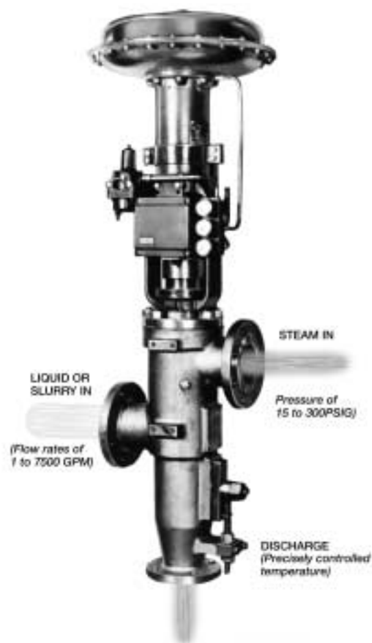
Figure 10-164. Direct steam heating of liquids with internal temperature control using variable orifice steam nozzle. (Used by permission: Bul. H 150. Hydro-Thermal Corp.)
