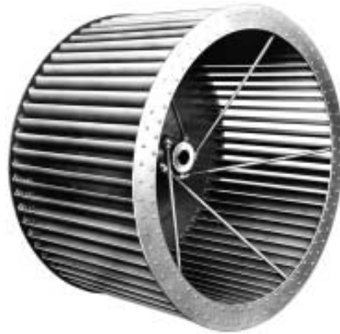
Figure 12-121. Single-width wheel (or impeller) with forward curved blades. (Used by permission: The Howden Fan Company.)
