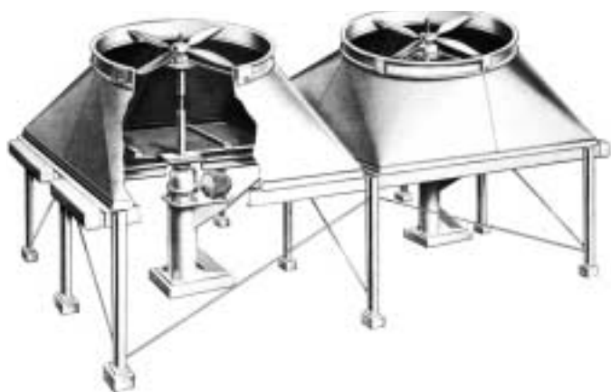
Figure 10-176. Typical induced draft air-cooled exchanger showing two exchanger sections and two fans. (Used by permission: Griscom-Russell/Ecolaire Corporation, Easton, PA.)
