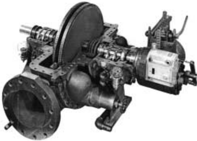
Figure 14-16B. View of Elliott YR Single Stage Steam Turbine, with top cover removed. (Used by permission: ©Elliott Co.)
