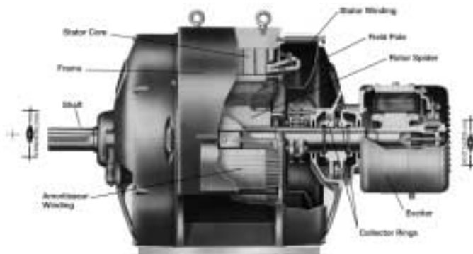
Figure 14-1A. A six-pole (1,200 rpm at 60 cycles) synchronous motor with direct-connected exciter. (Used by permission: E-M Synchronizer , Issue 200 SYN-42, ©1955. Dresser-Rand Company.)
