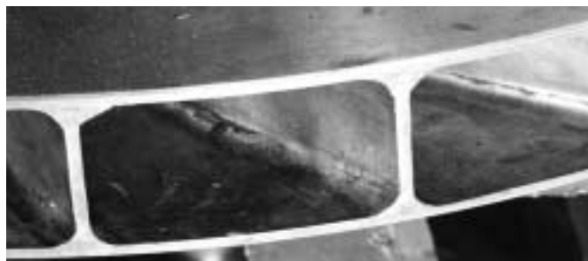
Figure 12-46D, Part 2. Close-up welding of section of welded impeller. (Used by permission: Elliott® Company.)
