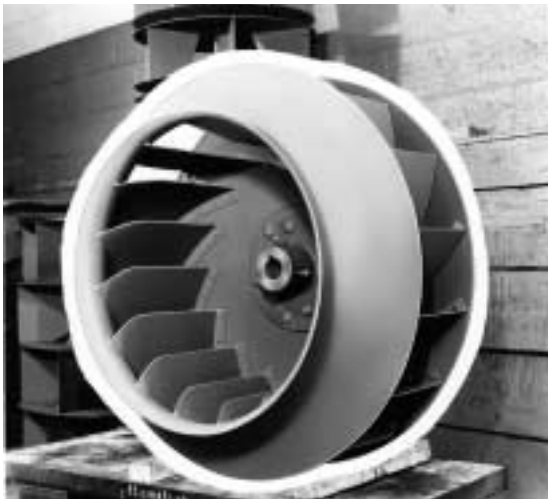
Figure 12-120A. Backwardly curved blades, Class 1 rotor. (Used by permission: The Howden Fan Co.)
