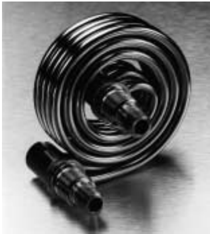
Figure 10-9C. Coil Assembly for bare tube Heliflow® exchanger. Tube sizes range from 1/4 - 3/4 in. O.D. Tube-side manifold connections are shown for inlet and outlet fluid. (Used by permission: Graham Manufacturing Company, Inc., Bul. HHE-30 © 1992.)
