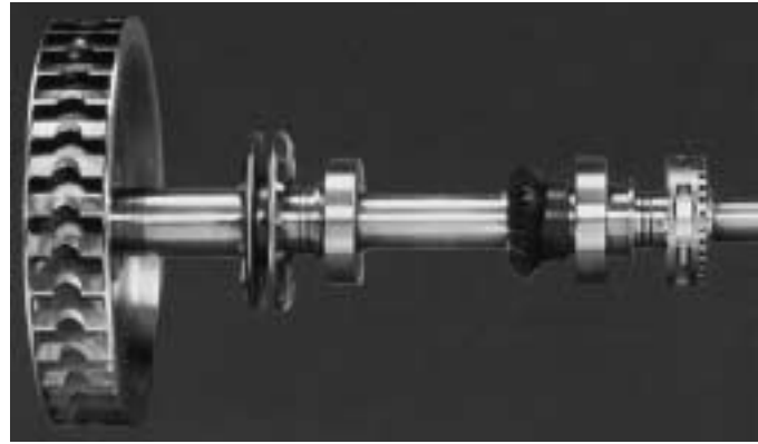
Figure 14-16C. Single Stage Steam Turbine Rotor: The GLT turbine features an overhung solid wheel that eliminates bearing box alignment problems and costs associated with installing steam separators or moisture traps commonly required for quick start applications. This overhung arrangement requires only one packing box, reducing the gland maintenance costs and potential leakage by half. (Used by permission: Bul. 8902-GLT.Dresser-Rand Company.)
