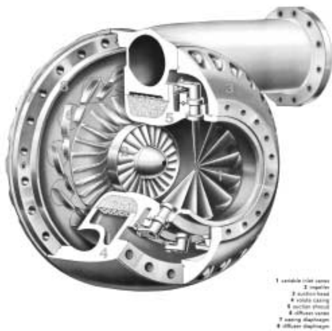
Figure 12-44B. Single-stage centrifugal compressor with variable inlet vanes, diaphragm, and diffuser vanes illustrated. (Used by permission: Worthington Power and Fluids , V. 8., No. 2, Winter, 1965. ©Dresser-Rand Company. All rights reserved.)
