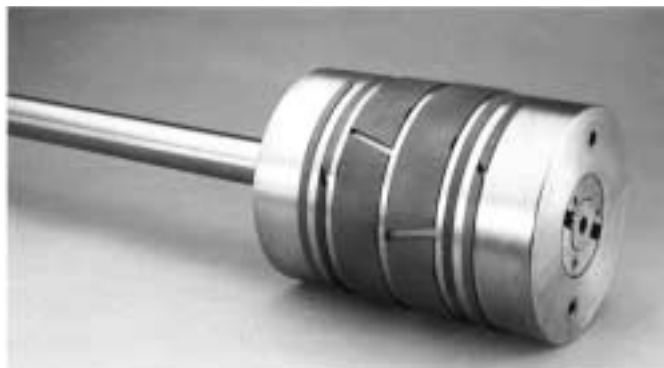
Figure 12-8. Pistons and rings. Lubricated and nonlubricated pistons with PTFE or other composite materials for the piston and rider rings. These designs prevent piston-to-bore contact and provide reliable service life, particularly during possible periods of lubrication interruption. (Used by permission: Bul. 85084, ©1992. Dresser-Rand Company.)
