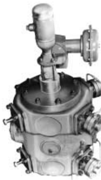
Figure 12-31A. Pneumatically operated clearance bottle. (Used by permission: Bul. 9-201B, ©1991. Cooper-Cameron Corporation. All rights reserved.)
