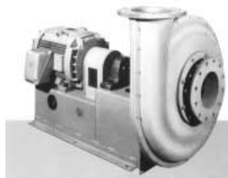
Figure 12-150. This standard arrangement 8 cast iron (C.I.) "E" blower, with motor and coupling factory mounted, is fitted with optional flanged inlet and outlet and coupling guard. (Used by permission: Bul. FI-411C (11/90), ©1988. The Howden Fan Co.)
