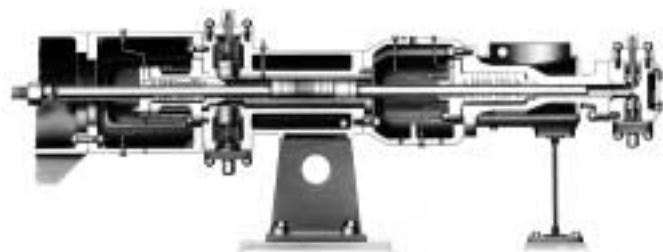
Figure 12-2O. Fourth- and fifth-stage cylinder assembly of 3,500 psig pressure hydrogen compressor. Opposed single-acting cylinders balance frame-bearing loading and minimize torque fluctuations. (Used by permission: Dresser-Rand Company.)
