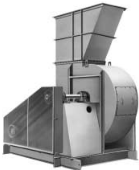
Figure 12-126. Evase duct attachment on fan discharge to improve the regain of static pressure. Fans can be purchased with or without the evase section. (Used by permission: Bul. 331, ©1992. The New York Blower Co.® For more information, contact the company at www.nyb.com.)
