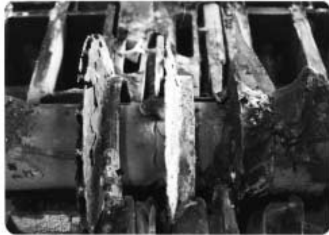
Figure 12-42. Results of internal chlorine gas fire and extensive corrosion in centrifugal compressor. Middle section of shaft with extensive damage to loss of center compression wheels. Note that ferric chloride is present.
