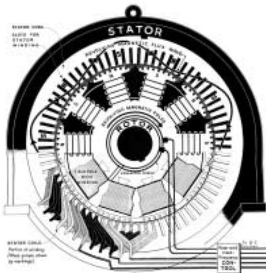
Figure 14-1B. Electrical connections in synchronous motors. (Used by permission: E-M Synchronizer , Vol. 7, No. 1, ©1944. Dresser-Rand Company.)
