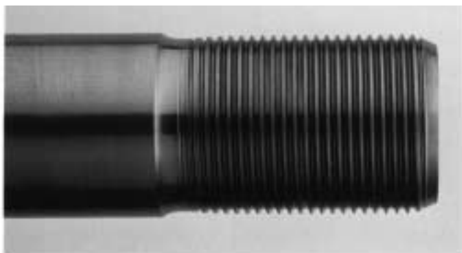
Figure 12-7. Piston rods. Precision-manufactured rolled threads and induction hardening provide high fatigue strength and long life in heavy duty service. Standard rod material is AISI 4142 carbon steel; other materials are available as required. Tungsten carbide coatings are also available for maximum surface hardness. Pistons are locked securely onto the rods. For higher pressure, smaller bore cylinders, the piston may be integral with the rod. (Used by permission: Bul. 85084, ©1992. Dresser-Rand Company.)
