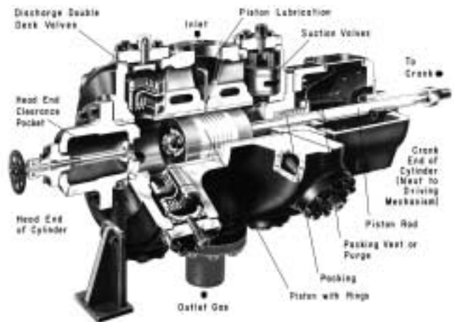
Figure 12-2B. Cut-a-way view of typical high-pressure gas cylinder showing double-deck feather valves in place. (Used by permission: Dresser-Rand Company.)
