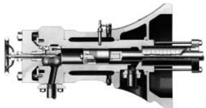
Figure 12-2K. Forged steel single-acting cylinder for 6,000 psi pressure. (Used by permission: Cooper-Cameron Corporation. All rights reserved.)
