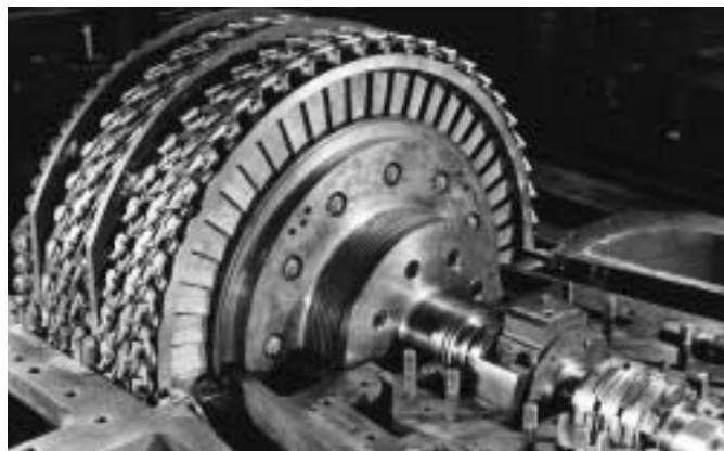
Figure 12-96. Stator blade control mechanism on four-stage axial compressor. (Used by permission: A C Compressor Corporation.)
