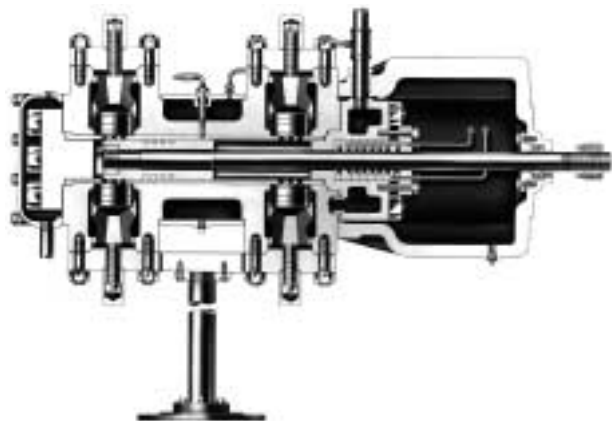
Figure 12-2N. Designed for working pressure up to 6,500 psi. A similar design cylinder is used for pressures in excess of 6,500 psi. Water cooled, forged steel, double-acting. (Used by permission: Dresser-Rand Company.)
