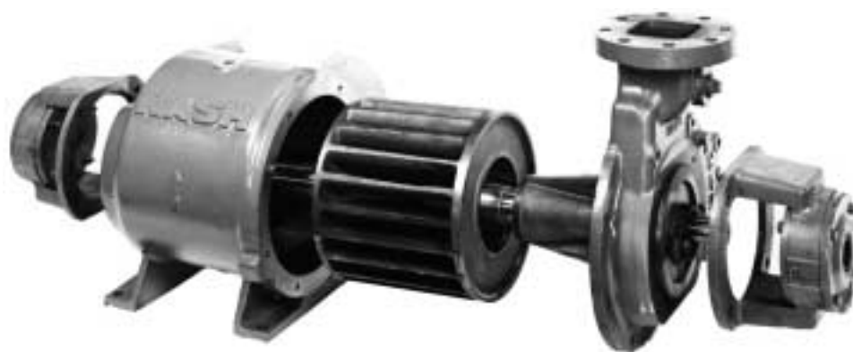
Figure 12-103B. A partly disassembled Nash liquid ring compressor view shows the pump body, the rotor, the cone, and the separate bearing blocks. (Used by permission: Bul. 778-A2/89, p.5. ©Nash Engineering Co.)
