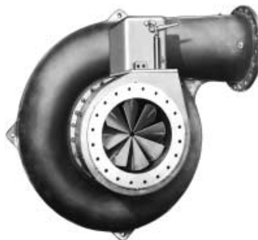
Figure 12-48B. Single-stage blower with automatically controlled inlet vaness. (Used by permission: A C Compressor Corporation.)
