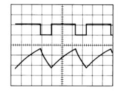
Top Trace: Output 5V/Div. Bottom Trace: Capacitor Voltage 1V/Div.
