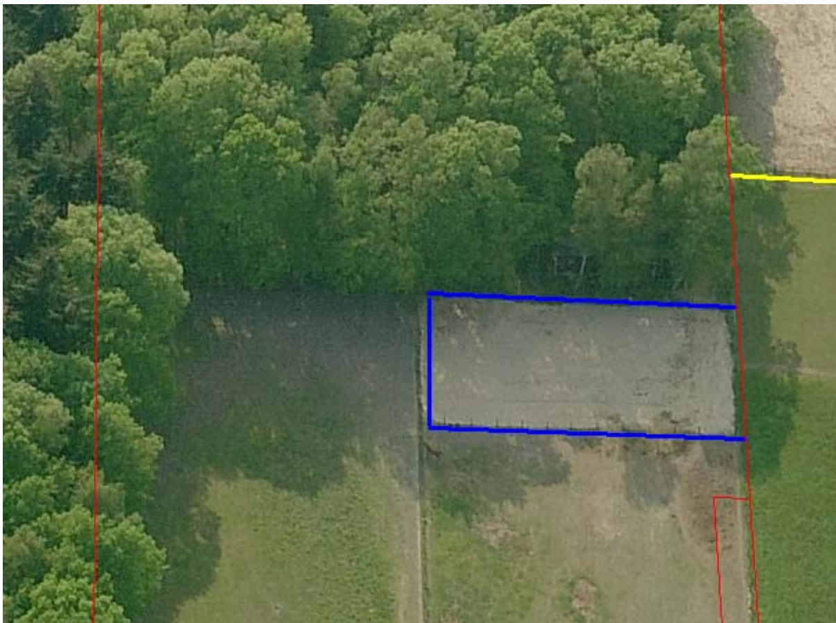
Figure 8, Identification of preliminary boundaries (blue) in oblique image. Existing cadastral boundaries are shown in red.
