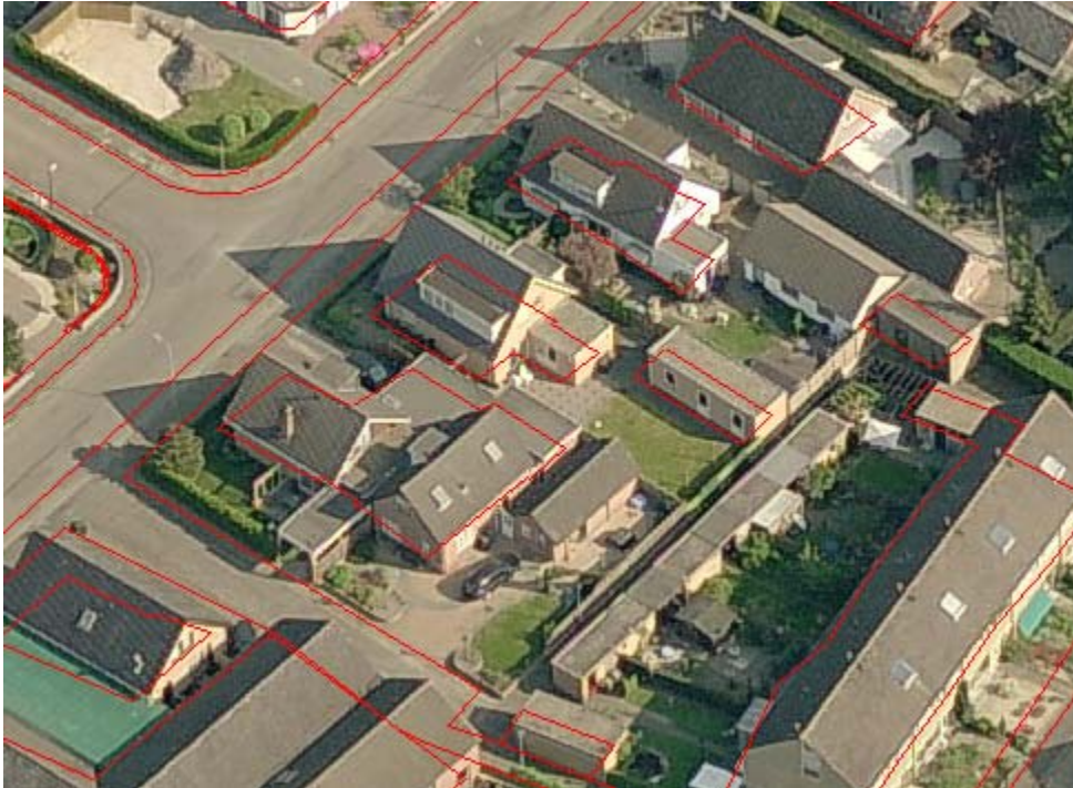
Figure 6, Projection of GBKN lines into oblique image.
