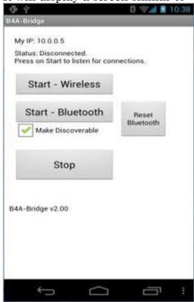
You should choose either **Start - Wireless** or **Start - Bluetooth** depending on the working mode. The **Make Discoverable** checkbox will make your device Bluetooth discoverable for 5 minutes. This is only needed if the device and computer weren't paired before.
