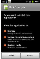
**Note**: the Bluetooth permission and Internet permission are automatically added in debug mode. Click on **Install**.
