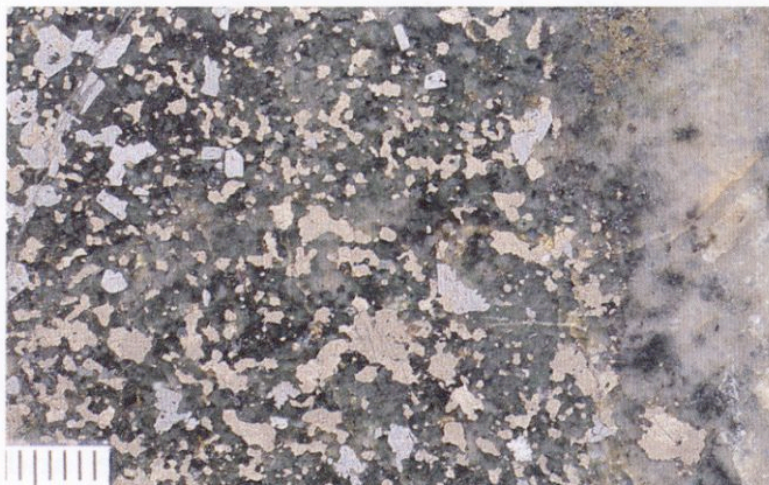
Figure 53 Abundant pyrrhotite (bronze) and arsenopyrite-loellingite (white) dissemination near mineralised quartz vein (on right) in the lower-granulite facies metasedimentary host rock at Griffin's Find. Silicates are plagioclase, quartz, diopside and hypersthene. Yellow specks are reflections of light from
