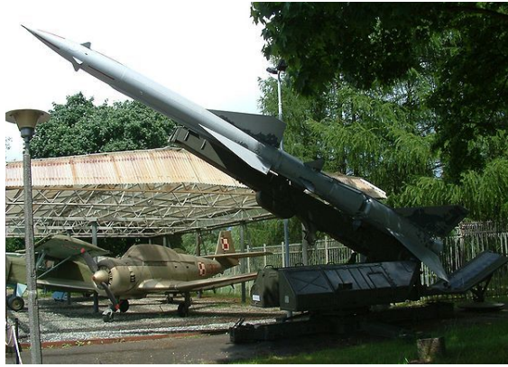
S-75 Dvina with V-750V 1D missile (NATO SA-2 Guideline) on a launcher. An installation similar to this one shot down Major Anderson's U-2 over Cuba.
