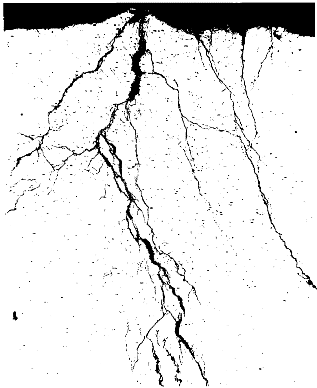
Figure 18. Section of Austenitic Stainless Steel Vessel Section Damaged by Severe Chloride Stress Corrosion Cracking (Etchant: Glyceregia).
