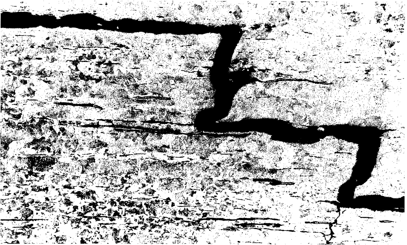
Figure 11. Characteristic Appearance of Cracks in Pump Shaft Failed in Fatigue (Etchant: 2 percent Nital).
