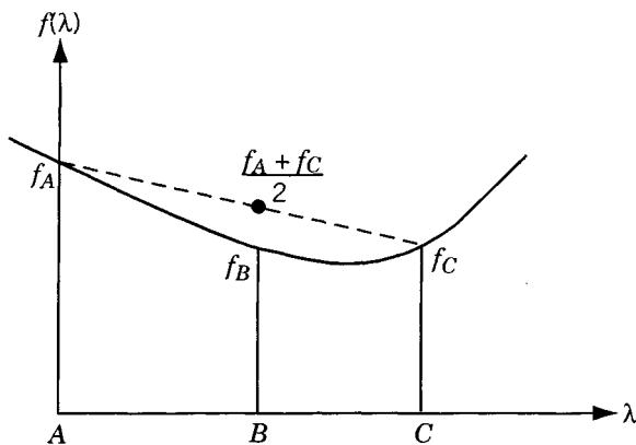
**Figure 5.12**  $f_B$  smaller than  $(f_A + f_C)/2$ .
