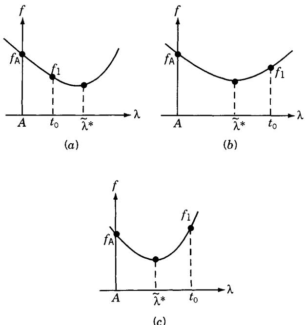
**Figure 5.13** Possible outcomes when the function is evaluated at  $\lambda = t_0$ : (a)  $f_1 < f_A$  and  $t_0 < \tilde{\lambda}^*$ ; (b)  $f_1 > f_A$  and  $t_0 > \tilde{\lambda}^*$ ; (c)  $f_1 > f_A$  and  $t_0 > \tilde{\lambda}^*$ .
