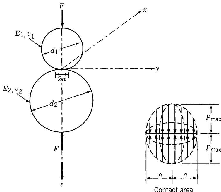
**Figure 5.2** Contact stress between two spheres.
