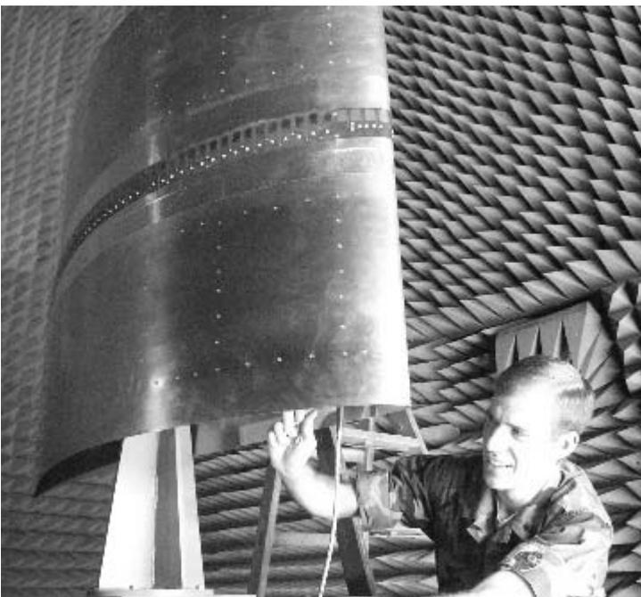
Figure 1.3. A microstrip array conformal to a wing profile in the test chamber. See also color insert, Figure 1. (Courtesy of Air Force Research Lab./Antenna Technology Branch, Hanscom AFB, USA.)
