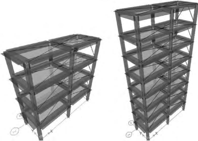
Figure 5.31 Torsionally unrestrained four-storey and eight-storey buildings.
