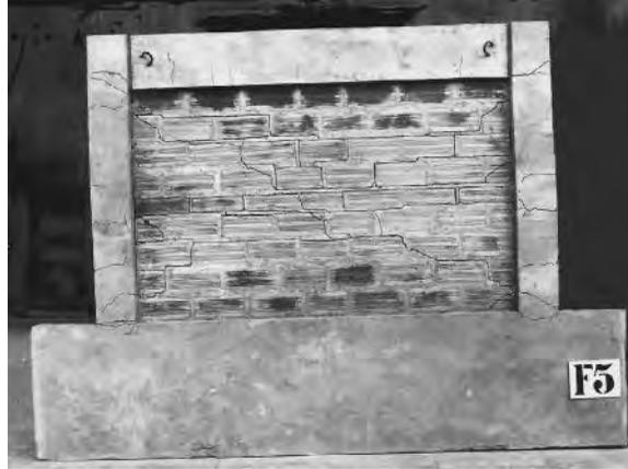
Figure 8.86 Failure mode of the infilled frame F5. (Adapted from Stylianidis, K. 2012. *Journal of O.C.B.T.*, 6, 194–212.)
