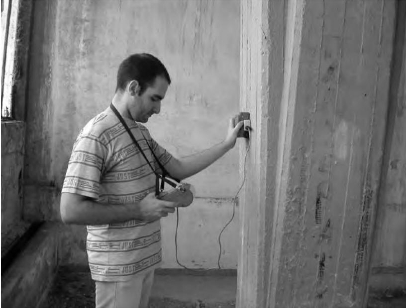
Figure 14.13 Electromagnetic steel detecting (MELISSARI Complex, Thessaloniki).
