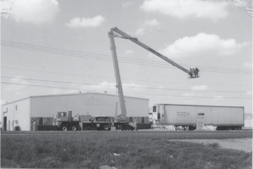
Figure 4-17. Insulated Bucket Vehicle.
