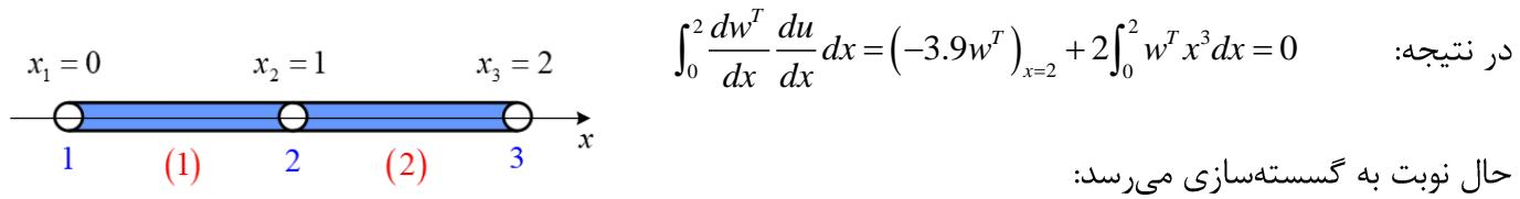
$$\int_{x_1}^{x_2} \frac{d(N\tilde{w})^T}{dx} \frac{d(N\tilde{u})}{dx} dx = (-3.9(N\tilde{w})^T)_{x=2} + 2 \int_{x_1}^{x_2} (N\tilde{w})^T x^3 dx = 0$$
