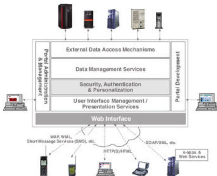
Figure 3.1: Basic, first-cut architectural framework for contemporary corporate portals.
