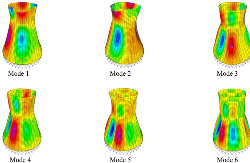
**Figure 4.** Variation of Deformed Shape CSA Mode 1,2,3,4,5,6
