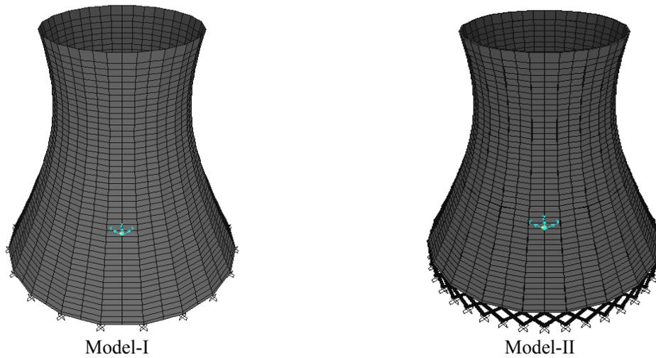
**Figure 2.** FBA&CSA Models of cooling towers
