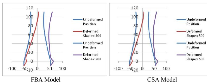
**Figure 5.** Radial displacements along the height of the tower for FBA, CSA
