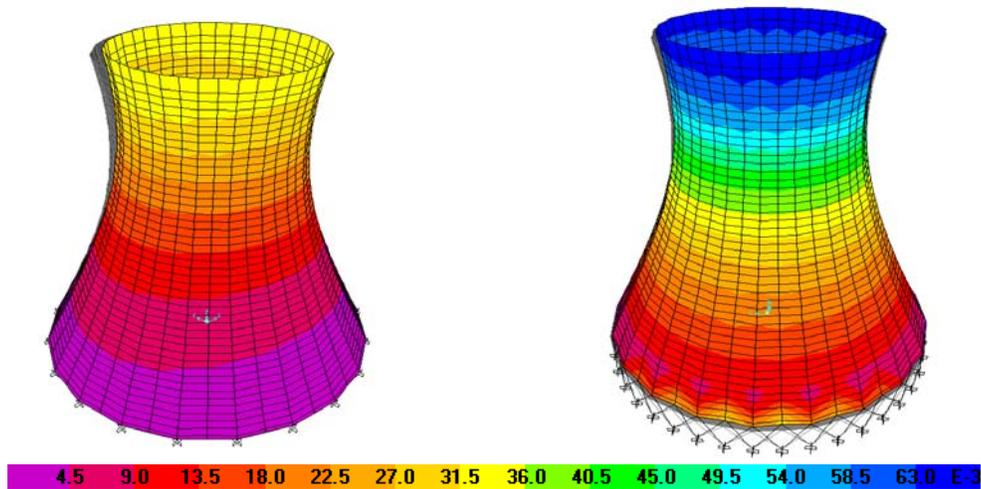
**Figure 6.** 3D Modeling of Radial displacements along the height of the tower for FBA, CSA
