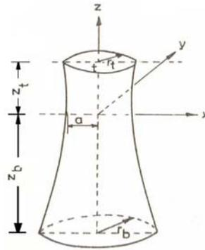
**Figure 1.** Cooling tower geometry (After Fonder and Clough, 1973)
