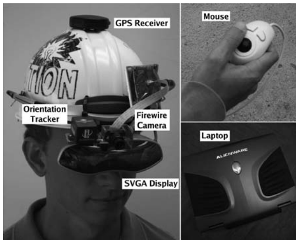
Fig. 2. Our wearable system hardware. An Alienware Area-51 m5500 laptop (worn in a backpack), an SVGA Sony Glasstron PLM-S700E display, a Point Grey Firefly firewire camera, An InterSense InertiaCube2 orientation tracker, a Garmin GPS 18 receiver, and an ErgoTouch RocketMouse.
