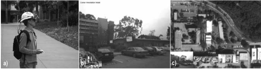
Fig. 1. A wearable system for outdoor annotation. Left to right: (a) A user wearing the system to annotate an outdoor scene. (b) The user's first-person view, showing the scene from the ground and the visible annotations. (c) The user's overhead view, showing an aerial photograph of the local region with the user's position and placed annotations overlaid.
