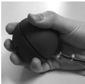
Fig. 4. The iOrb, an interaction device specifically designed for mobile AR users, unifies command input and 3D spatial selection at a distance through raypicking.
