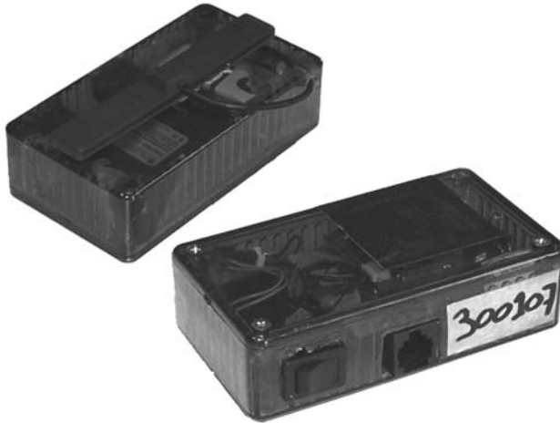
Fig. 5. BPS 2.0 tracking boxes (12 x 6.5 x 3.6 cm). On the one in front the connection for the battery loader or the optional external power source can be seen. On top of the other box, the GPS antenna is visible.
