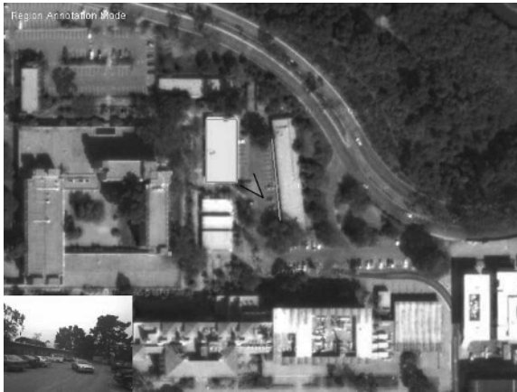
Fig. 4. The aerial photograph view from within the system. In the lower left corner, an insert of the video feed from the head-worn camera can be seen. The user's position and orientation are represented on the photograph with a small cone avatar. A small set of features have already been annotated – two corners (the green points), one edge (the green line), and one region (the transparent green rectangle).
