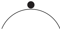
Fig. 3.4 A schematic illustration of an unstable fixed point. The marble is at an equilibrium, or fixed, position. However, a small perturbation will cause the marble to move away from the fixed point. This type of a fixed point is also known as a repellor.
