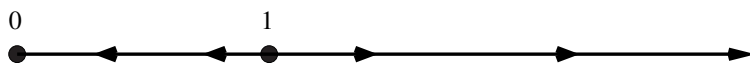
Fig. 3.1 The phase line for the function f(x) = x^2 , for non-negative x . Zero and 1 are fixed points. Seeds less than 1 approach 0. Seeds greater than 1 tend toward infinity.
