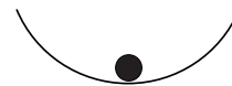
Fig. 3.5 A schematic illustration of a stable fixed point. The marble is at an equilibrium, or fixed, position. A small perturbation will cause the marble to move back toward the fixed point. This type of a fixed point is also known as an attractor.
