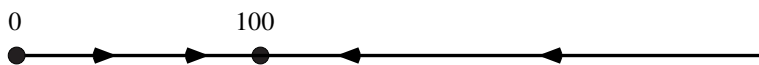
Fig. 29.3 The phase line for the differential equation of Eq. (29.1). There is an attracting fixed point at P = 100 .
