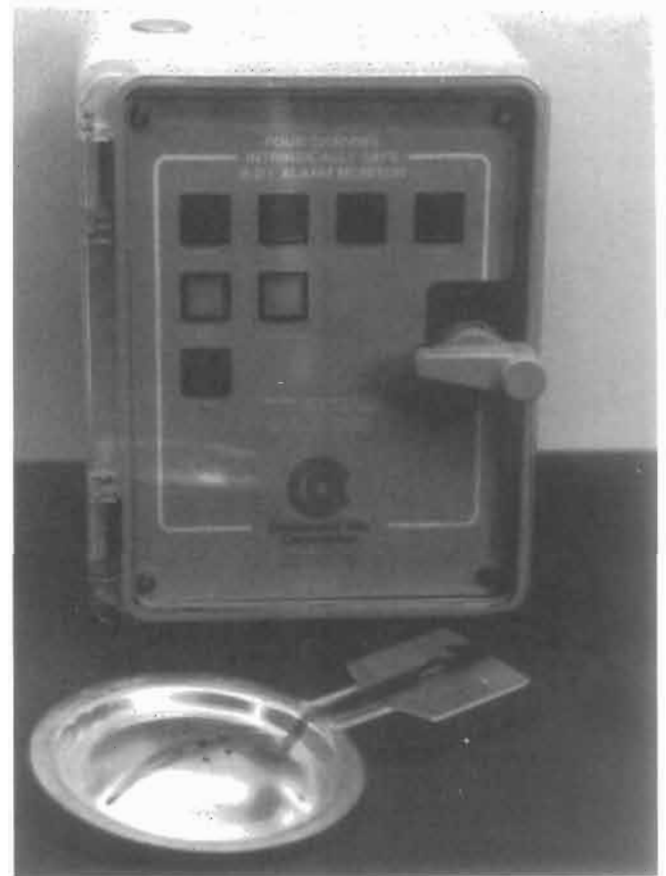
Figure 7-8L. Rupture disk indicator alarm strip breaks when rupture disk breaks and alarms to monitor. FM system approved. By permission, Continental Disc Corporation.
