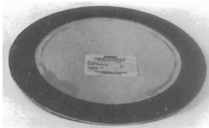
Figure 7-8I. Flat disk used for low pressure and for isolation of corrosive environments. Usual pressure range is 2 to 15 psig with \pm 1 psi tolerance. Stainless steel disk with Teflon® seal is usually standard. By permission, Fike Metal Products Div., Fike Corporation. Catalog 73877-1, p. 35.
