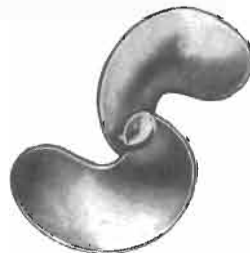
Figure 5-5Q. Weedless propeller. Handles long fibrous materials that would become entangled in the ordinary propeller. Courtesy of Lightnin (formerly Mixing Equipment Co.), a unit of General Signal.
