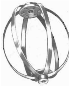
Figure 5-5K. Plain cage beater. Imparts a cutting and beating action. It is usually combined with a standard propeller, which supplies movement in the mix. Courtesy of Lightnin (formerly Mixing Equipment Co.), a unit of General Signal.
