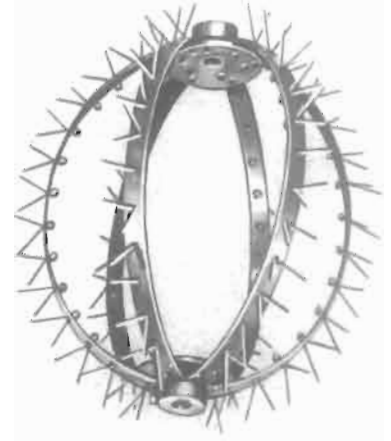
Figure 5-5L. Studed cage beater. Enormous contact area gives extremely violent cutting and shredding action to certain emulsions, pulps, etc. Courtesy of Lightnin (formerly Mixing Equipment Co.), a unit of General Signal.
