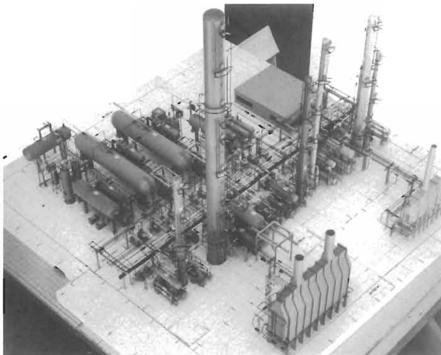
Figure 1-16B. Detailed layout and piping model for a refinery unit. Courtesy of Socony Mobil Oil Co. Inc.
