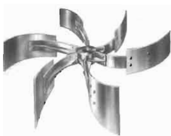
Figure 5-5T. Standard six-blade vertical curved blade turbine impeller. Gives good efficiency per unit of horsepower for suspensions, mixing fibrous materials. Gives high pumping capacity. Courtesy of Philadelphia Gear Corp.
