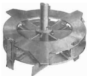
Figure 5-5U. Shrouded turbine for high pumping capacity. Usually used with low static heads, creates minimum of direct shear. Courtesy of International Process Equipment Co., Div. of Patterson Foundry and Machine Co.
