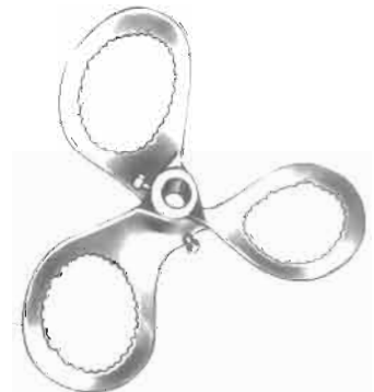
Figure 5-5R. Cut-out propeller. Displaces a small amount of liquid combined with a high rate of shear for shredding, breaking up pulps, etc. Courtesy of Lightnin (formerly Mixing Equipment Co.), a unit of General Signal.
