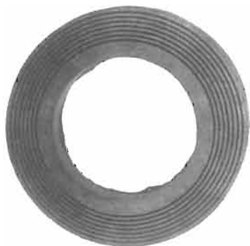
Figure 7-9A. Non-metal frangible disk. Ruptured disk showing complete breakout of membrane. Courtesy of Falls Industries, Inc.
