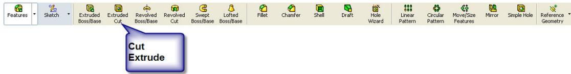
15. Cut Extrude Blind into the cube 20mm.
