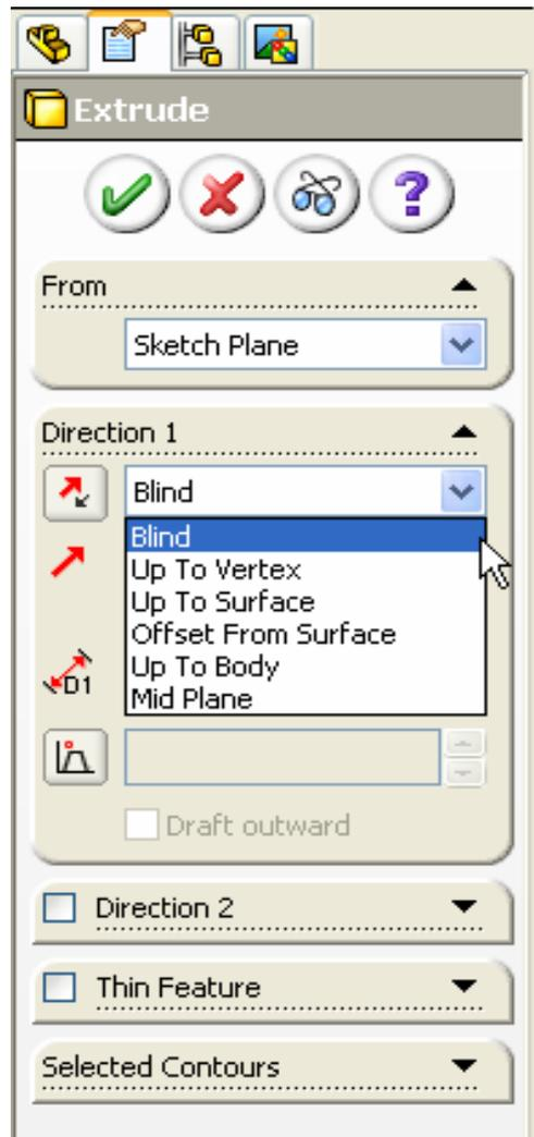
Design Intent at extrusion stage.
