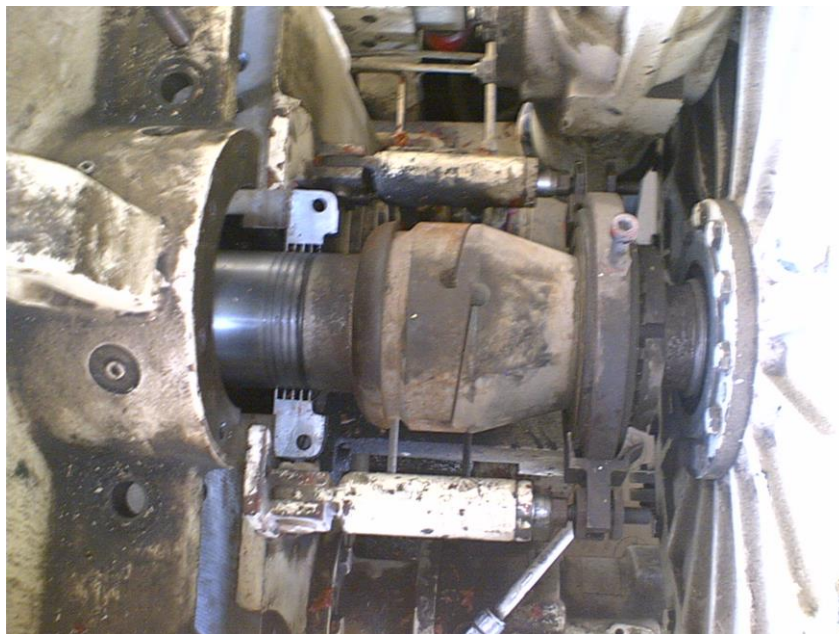
Figure 39: A One Direction Ratchet Clutch (Picture Belongs to Unit 120 of Phase 2&3 of S.P.G.C.)
