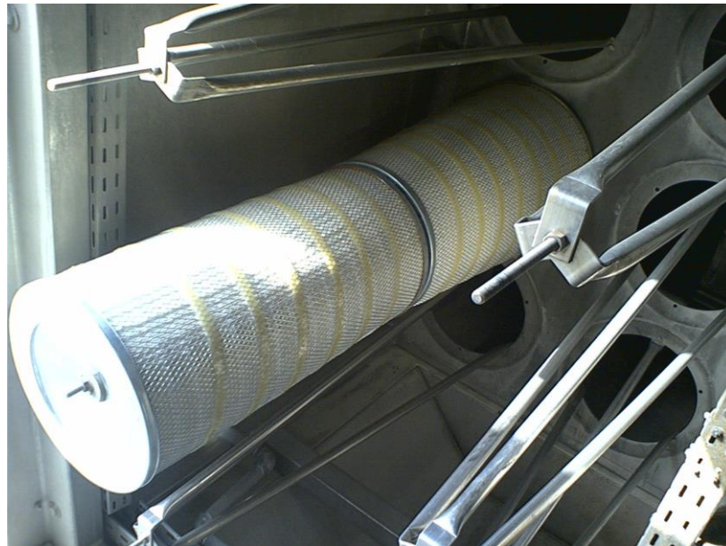
Figure 5: A Self-Clean Filter Element (Picture Belongs to Unit 106 of Phase 2&3 of S.P.G.C.)
