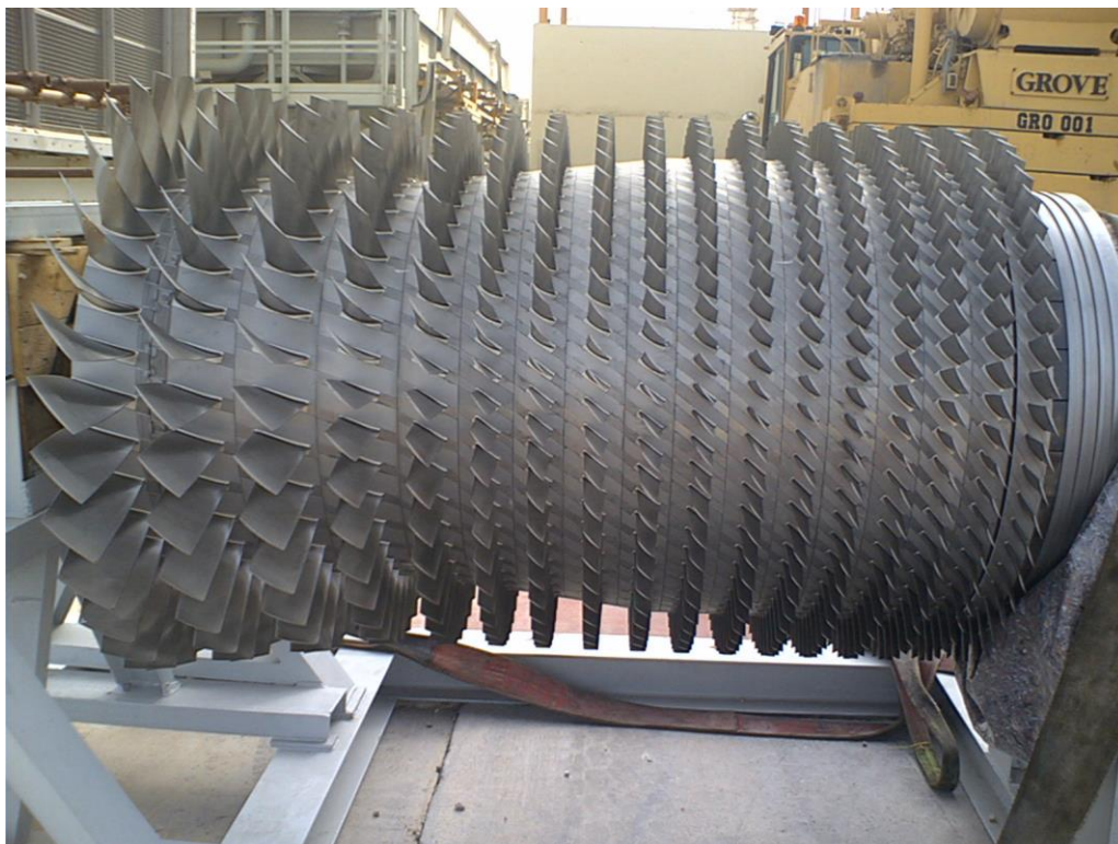
Figure 14: A Seventeen Stage Axial Compressor Rotor (Picture Belongs to Unit 120 of Phase 2&3 of S.P.G.C.)
