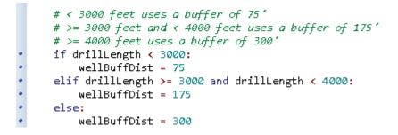
Next, buffer the input feature class by the determined well buffering distance. Store the output in a file named **SelectionBuffer**, and store it in a separate workspace, **C:\EsriPress\GISTPython\ MyExercises\Scratch\TemporaryStorage.gdb**.
