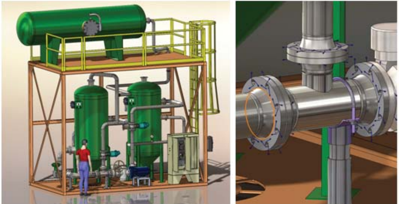
FIGURE 6. A PIPE ROUTE CONTAINS MANY BOLTED FLANGES, MODELED WITH BOLT CONNECTORS SHOWN IN BLUE (RIGHT).
