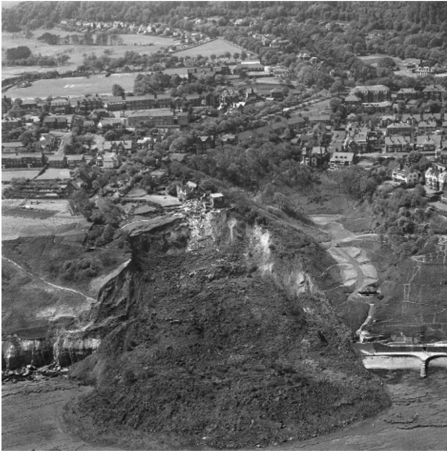
Figure 12.7 Rotational slope failure at Holbeck, Yorkshire.
